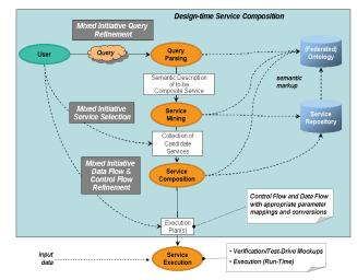
**Figure 1:** Simplified Workflow – Mixed initiative design-time functionality supports users as they refine the specification of composite services, identify and select relevant services and compose them. Actual workflows often involve multiple iterations.
