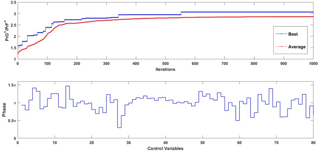
Fig. 8. Experimental result on the femtosecond laser control system for optimizing the ratio between the products  $\text{PrO}^+$  and  $\text{PrF}^+$  using MS\_DE when no constraint on the phase. (a) Ratio  $\text{PrO}^+/\text{PrF}^+$  vs iterations, where ‘Best’ represents the maximum fitness and ‘Average’ represents the average fitness of all individuals during each iteration. (b) Optimized phases of 80 control variables for the optimal result that corresponds to the maximum fitness.
