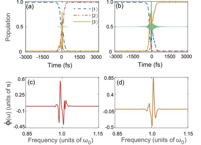
Fig. 4. Optimal population evolutions and spectral phases with  $\sigma = 50$   $\text{cm}^{-1}$ . The population evolutions of quantum state transfer to the target state (a)  $|2\rangle$  and (b)  $|3\rangle$  with laser pulses in green. The corresponding optimized spectral phases for (a) and (b) are shown in (c) and (d).
