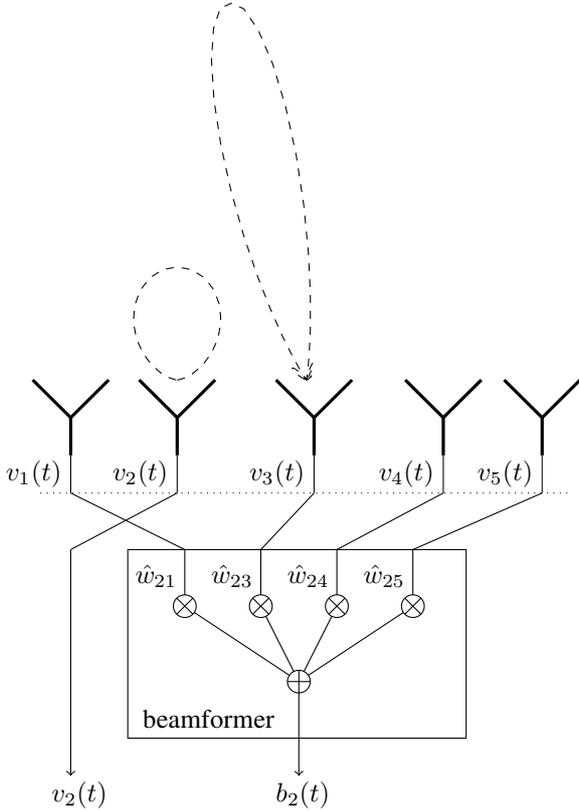
Fig. 1. Illustration of the cross-correlation between the voltage  $v_2$  and the beamformed voltage  $b_2$  used to determine the gain  $g_2$ . The dotted line and the dashed lines represent, respectively, the ADC output and the radiation patterns associated to  $v_2$  and  $b_2$ .
