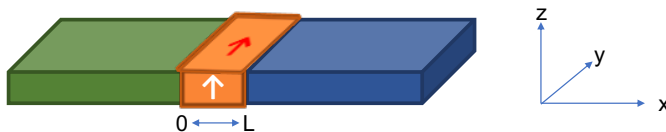
FIG. 1. Schematic representation of N-M-S junction with magnetic strips on top and side surfaces. The green region denotes the normal WSM-II, orange denotes the magnetic region, while the blue denotes the superconducting part of the junction. The magnetic strips induces the desired magnetization in the region 0 \leq x \leq L . The red and white arrows denotes the direction of induced magnetization along \hat{y} and \hat{z} respectively.
