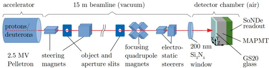
Figure 1: A schematic view of the experimental setup (not to scale). The accelerator (left) produced continuous beams of protons or deuterons with currents in the  $\sim$ nA range. The beams were transported and reduced in intensity via a beamline (middle) ending in a thin vacuum window. A detector chamber (right) operated at room temperature and pressure was positioned downstream of this window. The detector chamber contained a SoNDe module mounted on a motorized platform.
