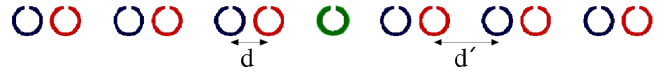
FIG. 1: (color online) Schematic of the topological \mathcal{PT} -metamaterial. The blue, red, and green split-ring resonator(s) have loss, gain, and neither gain nor loss, respectively. SRRs separated by center-to-center distance d ( d' ) are coupled magnetically and electrically through intra-dimer (inter-dimer) coefficients \lambda_M and \lambda_E ( \lambda'_M and \lambda'_E ), respectively.
