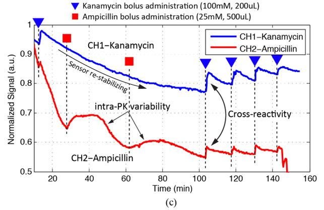
Fig. 5. (a) *in vivo* demonstration with a rodent model. (b) The photo of the implanted probe. (c) Measured responses of two aptamers.
