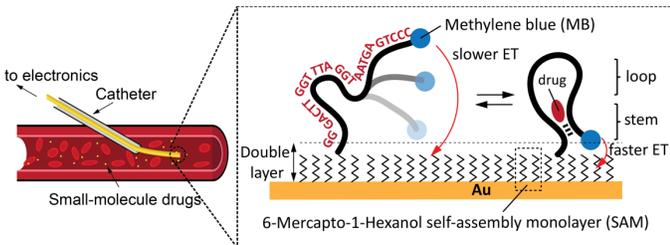
Fig. 2. The operation of structure-switching aptamer with and without the presence of the drug and its use in *in vivo* monitoring.
