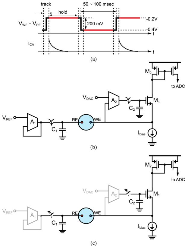
Fig. 8. (a) Proposed CA with sample-and-hold operation. (b) Simplified circuit schematics in the potential-tracking phase. (c) Simplified circuit schematics during the hold phase.
