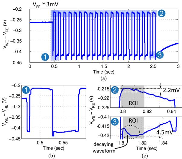
Fig. 14. (a) Measured electrode waveforms when interfacing with an aptamer device. (b) A zoom-in of the first pulse. (c) Waveforms during the hold phases.
