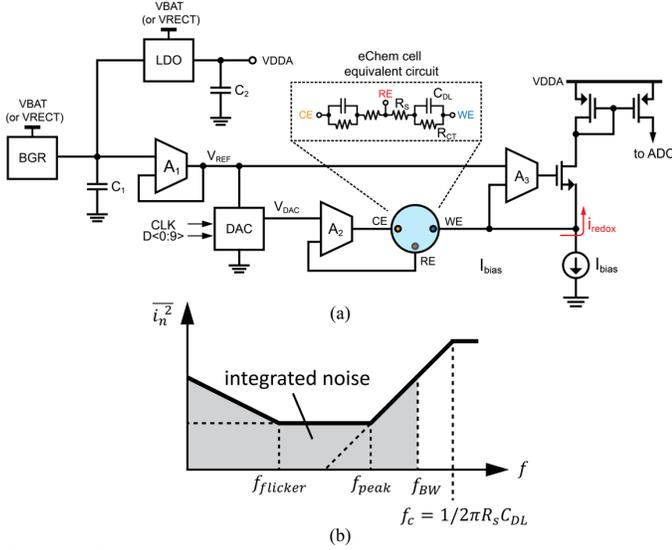
Fig. 7. (a) The system block diagram of a conventional electrochemical-sensing circuit. (b) PSD illustration of noise peaking.
