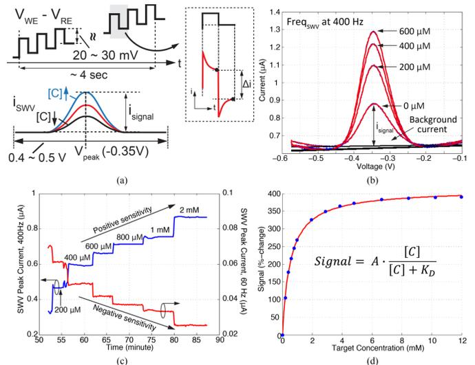
Fig. 3. (a) SWV operation. (b) SWV voltammograms at 400 Hz at different kanamycin concentrations. (c) Measured time-series at 400 and 60 Hz SWV frequencies. (d) Fitting of the binding curve with Langmuir isotherm model.
