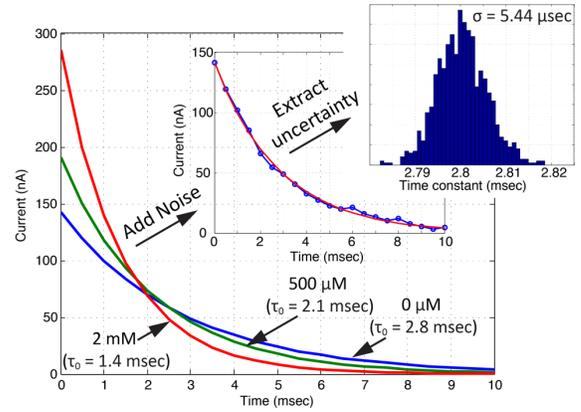
Fig. 6. Monte Carlo simulation for studying impact of electronics noise.
