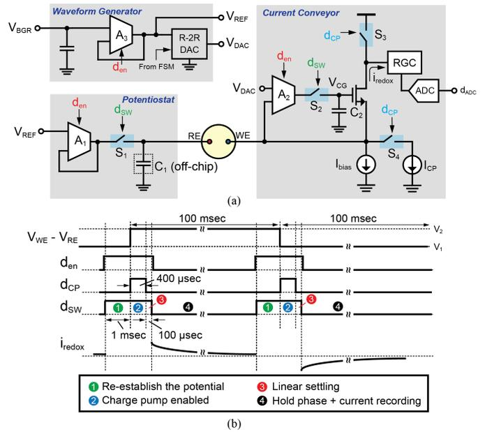
Fig. 9. (a) Complete circuit schematics. (b) Operational timing diagram.
