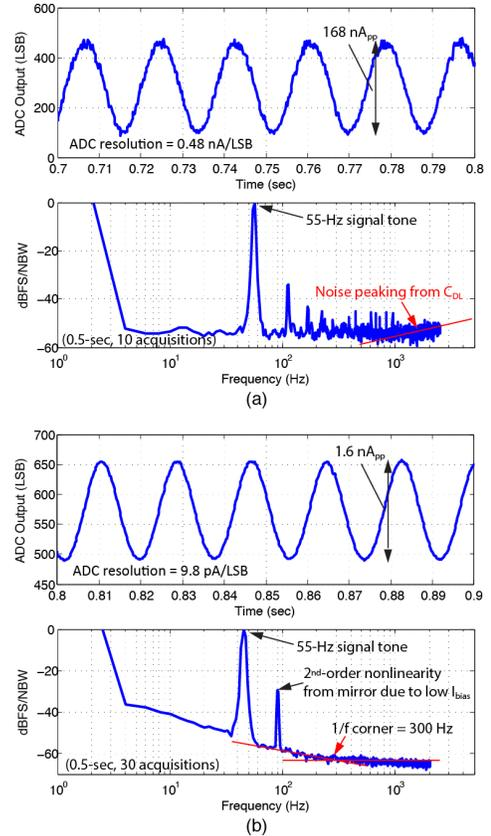
Fig. 13. Measured time-domain waveforms and PSDs with S/H: (a) disabled and (b) enabled.
