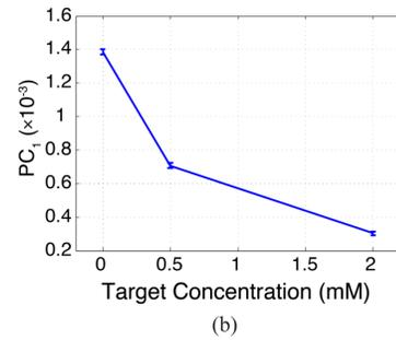
Fig. 17. Extracted principal component (a) vs. time and (b) vs. concentration. Error bar stands for one standard deviation.
