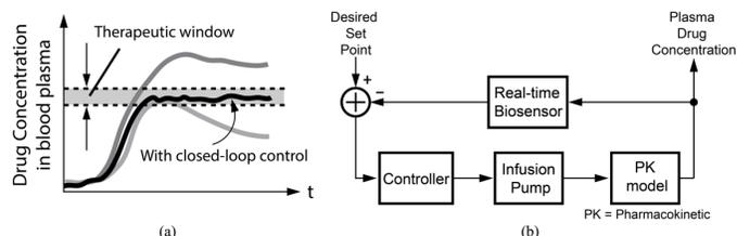
Fig. 1. (a) Real-time therapeutic drug monitoring enables precision drug dosing for optimal treatment outcome. (b) A generic closed-loop drug control system.
