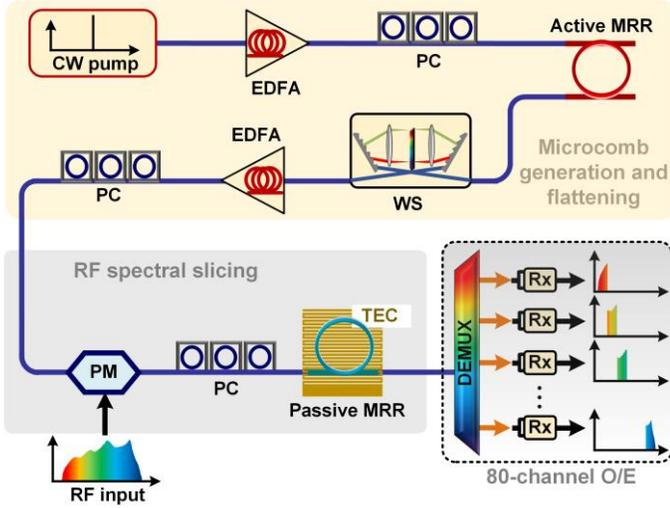
Fig. 1. Schematic diagram of the broadband RF channelizer based on a soliton crystal microcomb. EDFA: erbium-doped fibre amplifier. PC: polarization controller. MRR: micro-ring resonator. WS: Waveshaper. PM: phase modulator. TEC: temperature controller. DEMUX: de-multiplexer. Rx: Receiver.
