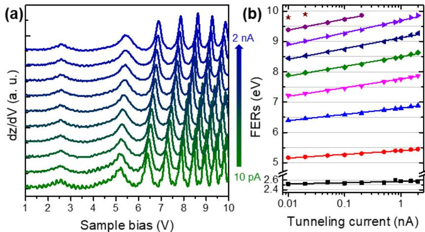
**Figure S6.** Stark shift in the FERs of TbAu<sub>2</sub>/Au(111). (a) A series of dz/dV spectra of TbAu<sub>2</sub>/Au(111) taken at the hill region under the tunneling current from 20 pA to 2.0 nA. The spectra are vertically shifted evenly for clarity. (b) Relations between the FERs and the tunneling current. The solid lines are the linear fit under the semi-log in the current axis.
