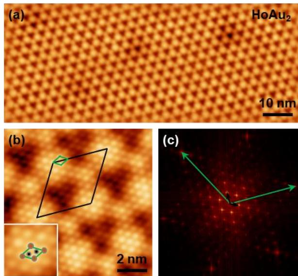
**Figure 3.** STM topographic images of  $\text{HoAu}_2$ . (a) Large-scale and (b) atomically resolved STM images of  $\text{HoAu}_2$  on  $\text{Au}(111)$ , respectively. Inset in (b) shows its zoom-in image, where the orange
