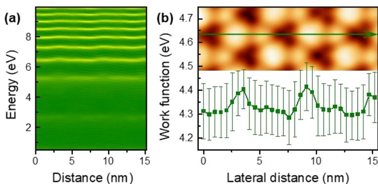
**Figure S7.** Surface work function of HoAu<sub>2</sub>/Au(111). (a) Line mapping of dz/dV spectra and (b) Surface work function profile along the green line in top panel of (b). The surface work function was obtained by fitting the dz/dV spectra in (a) according to the equation (1) in the main text.
