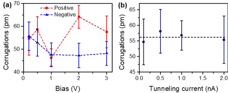
**Figure S2.** Bias-dependent height corrugations in TbAu<sub>2</sub>/Au(111). Relationships between the height corrugations and (a) sample bias, and (b) tunneling current. Tunneling condition for (a):  $I_{\text{set}} = 100$  pA, (b)  $V = 0.2$  V.
