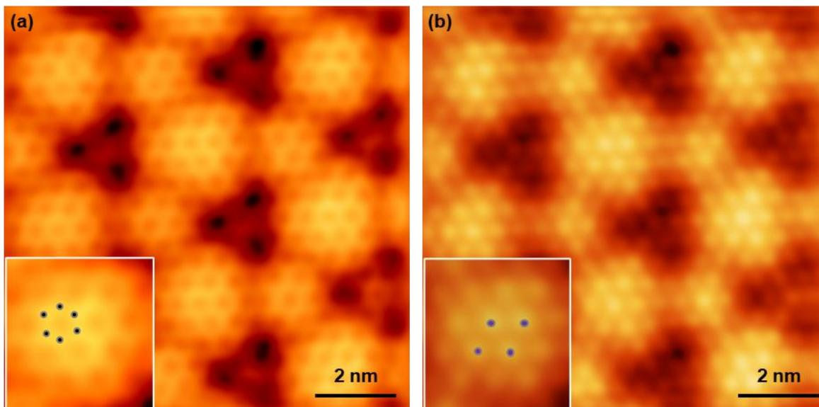
**Figure S1.** Atomic-resolution STM images of TbAu<sub>2</sub> monolayer on Au(111) under (a) 0.5 V and (b) -0.5 V, respectively. The insets show the zoomed-in images, showing honeycomb and triangular lattices, respectively. The tunneling current was set to be 2.0 nA for both (a) and (b).
