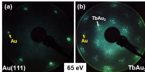
**Figure 2.** LEED patterns of (a) clean Au(111) and (b) TbAu<sub>2</sub>/Au(111).
