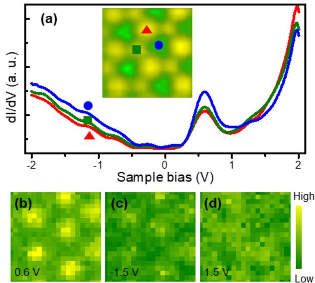
**Figure 5.** STS differential conductance spectra and mappings of  $\text{TbAu}_2/\text{Au}(111)$ . (a)  $dI/dV$  spectra of  $\text{TbAu}_2$  taken at three different regions (indicated in the inset STM image with area of  $9 \times 9 \text{ nm}^2$ ) within the unit cell of the moiré structure of  $\text{TbAu}_2$ . (b-d) Differential conductance mappings of  $\text{TbAu}_2$  at sample bias at 0.6 V, -1.5 V, and 1.5 V, respectively. The corresponding topographic
