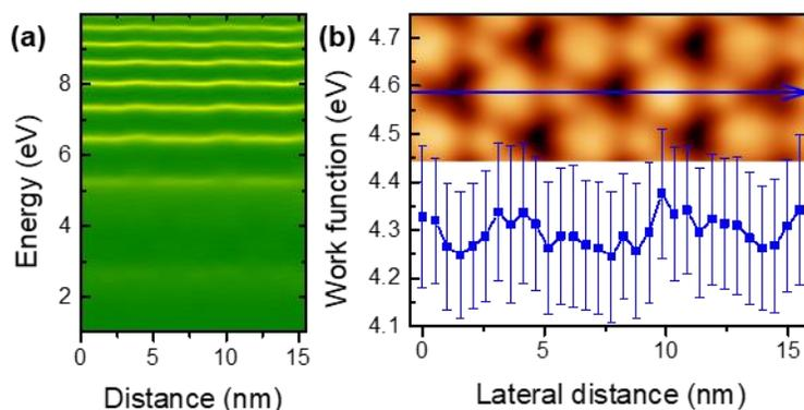
**Figure S8.** Surface work function of ErAu<sub>2</sub>/Au(111). (a) Line mapping of  $dz/dV$  spectra and (b) Surface work function profile along the green line in top panel of (b). The surface work function was obtained by fitting the  $dz/dV$  spectra in (a) according to the equation (1) in the main text.
