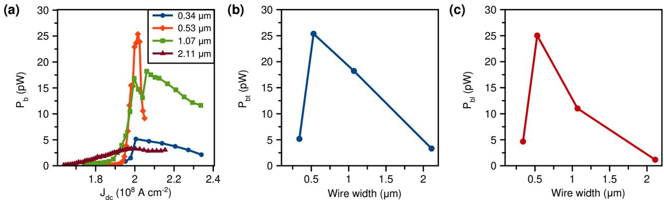
FIG. 3. (a) Integrated microwave power emitted by all bulk modes of the wire  $P_b$  versus bias current density  $J_{dc}$ . The data is shown for all four wires exhibiting bulk mode auto-oscillations. (b) Maximum value of the integrated microwave power emitted by all bulk modes of the wire  $P_{bt}$  as a function of the wire width. (c) Maximum integrated power of the largest-amplitude bulk mode  $P_{bl}$  as a function of the wire width.
