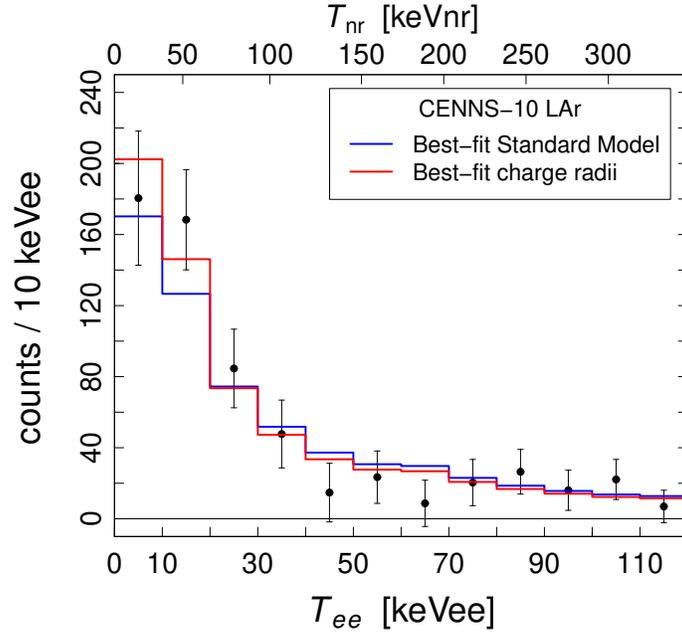
FIG. 6. Histogram representing the fits of the CENNS-10 data (black points with statistical error bars) with the Standard Model charge radii given in Eqs. (40) and (41) (blue histogram), and with the best-fit charge radii of the COHERENT Ar data analysis (red histogram).
