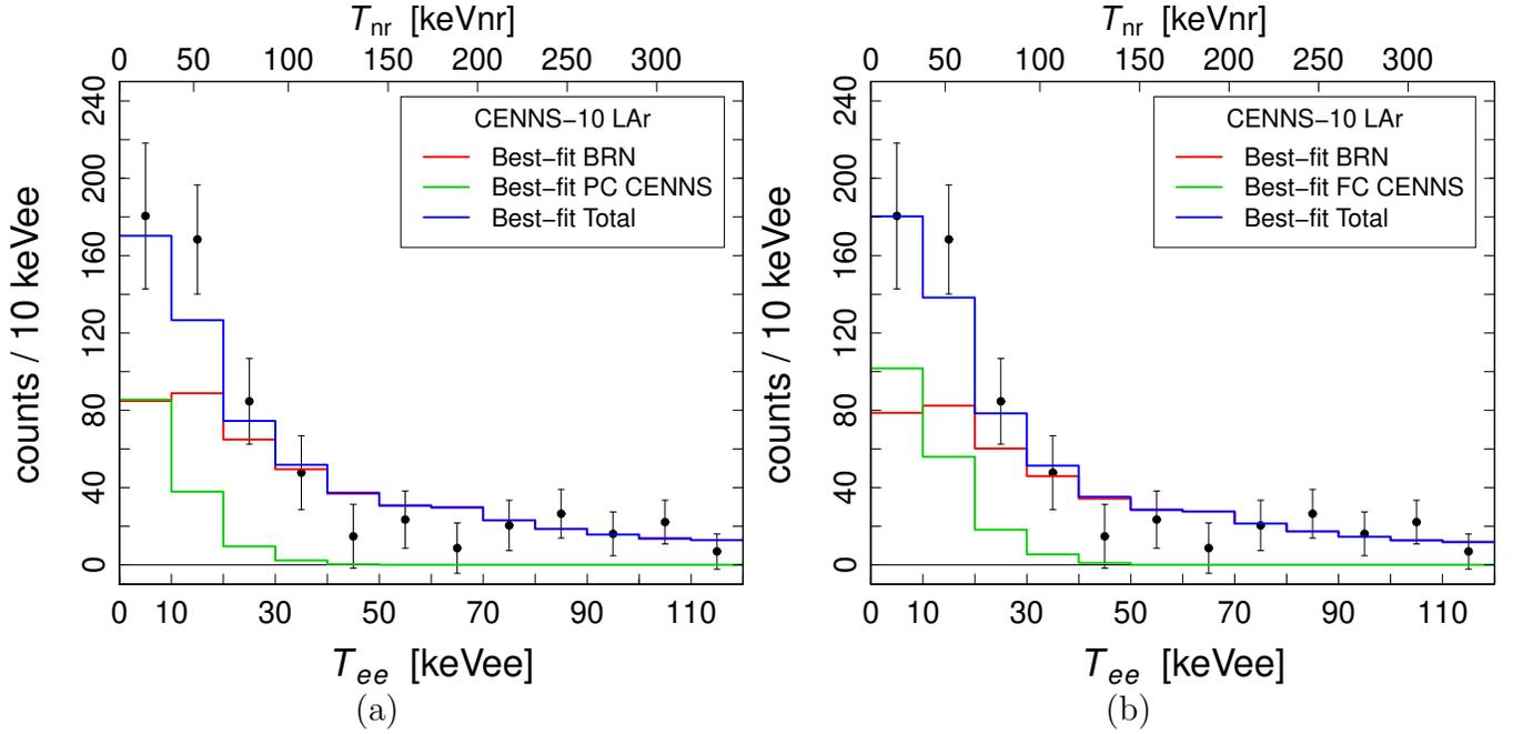
FIG. 1. Histograms representing the fits of the CENNS-10 data (black points with statistical error bars) in the case of (a) partial coherence (PC), with the neutron form factor corresponding to the minimal neutron distribution radius  $R_n = 3.45$  fm, and (b) full coherence (FC).
