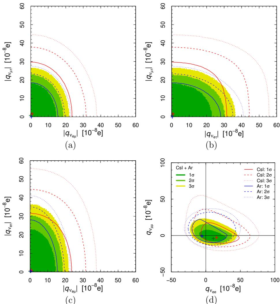
FIG. 8. Contours of the allowed regions in different planes of the neutrino electric charge parameter space obtained with fixed  $R_n$  obtained from the analysis of COHERENT CsI data (red lines), from the analysis of COHERENT Ar data in this paper (blue lines), and from the combined fit (shaded green-yellow regions). The crosses with the corresponding colors indicate the best fit points.
