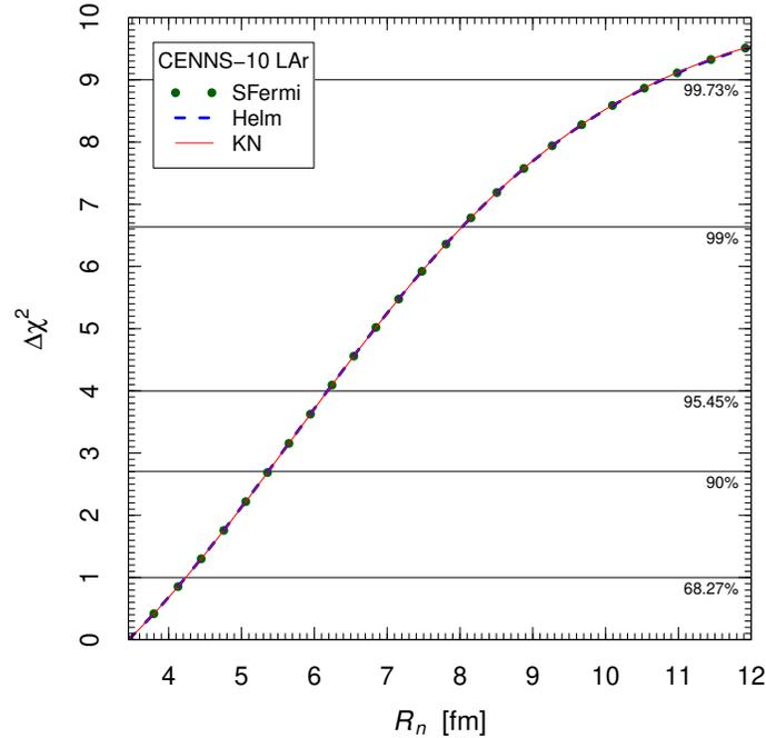
FIG. 2.  $\Delta\chi^2 = \chi_S^2 - (\chi_S^2)_{\min}$  as a function of the rms neutron distribution radius  $R_n$  of  $^{40}\text{Ar}$  obtained from the fit of the data of the CENNS-10 experiment. The three curves correspond to the symmetrized Fermi [26] (SFermi), Helm [27] (Helm), and Klein-Nystrand [28] (KN) form factor parameterizations.
