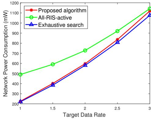
Fig. 4: Network power consumption versus target data rate.
