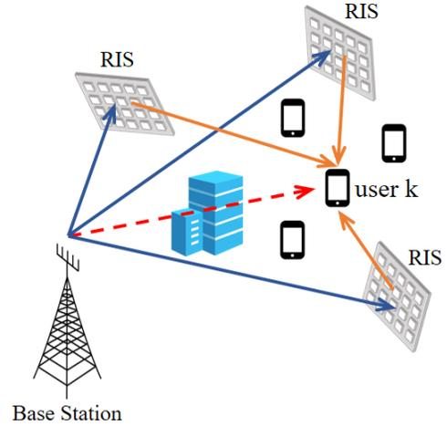
Fig. 1: An illustration of a multi-RIS-assisted multi-user MISO downlink cellular network.
