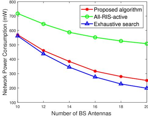
Fig. 3: Network power consumption versus number of BS antennas.
