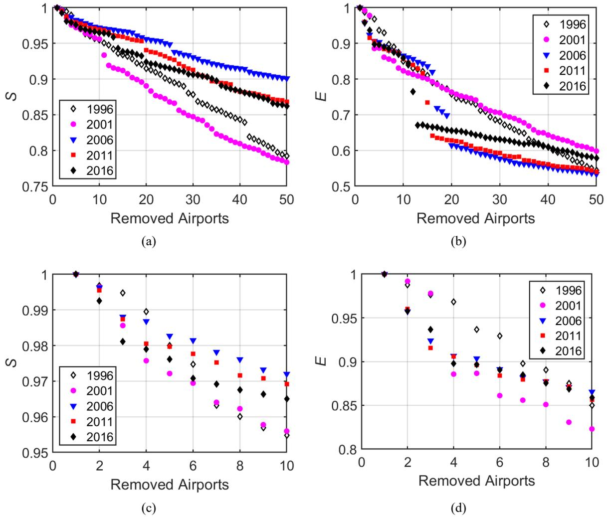
Figure 10. The evolution of the network's largest connected component  $S$  and efficiency  $E$  as a function of nodes removed. Parameters  $S$  and  $E$  are normalized by their respective maximum value observed for each specific year.
