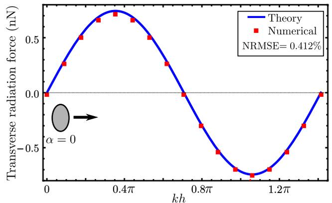
FIG. 8. Numerical and theoretical calculations of the transverse radiation force ( $F_{x'}^{\text{grad}}$ ) on a spheroidal particle as a function of the scaled distance  $kh$ . The particle (gray ellipse) has a geometric parameter of  $\xi_0 = 1.3181$  with orientation  $\alpha = 0$ . The simulational parameters are presented in Table I.
