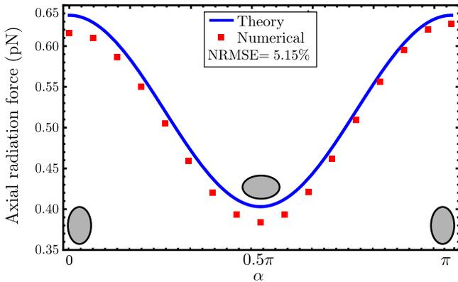
FIG. 9. The axial radiation force ( $F_z^{\text{sca}}$ ) at a pressure node versus particle orientation. The particle (gray ellipses) has a geometric parameter of  $\xi_0 = 1.3181$ . The simulational parameters are surveyed in Table I.
