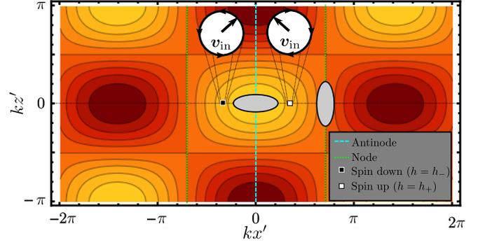
FIG. 4. The amplitude (real part) of the incoming wave in Eq. (28). The equilibrium orientation of the spheroidal particle (gray ellipses) are illustrated in a node ( $\alpha = 0$ ) and antinode ( $\alpha = \pi/2$ ). The fluid velocity polarizabilities are shown when  $h = h_+ = \sqrt{2}\pi/4k$  (spin up) and  $h = h_- = -\sqrt{2}\pi/4k$  (spin down). Color legend:  $p_0$  (bright yellow) and  $-p_0$  (dark red).
