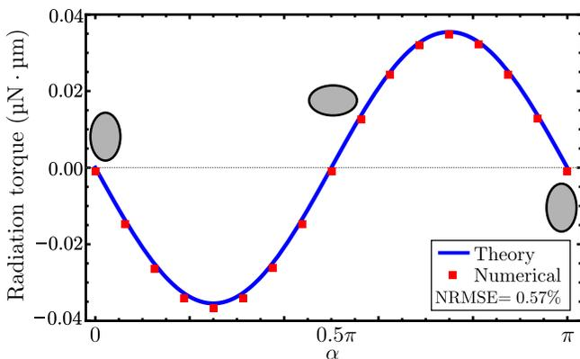
FIG. 10. The theoretical and numerical results of the radiation torque versus orientation angle  $\alpha$ . The particle (gray ellipses) has a geometric parameter of  $\xi_0 = 1.3181$  and is trapped in a pressure node. The simulational parameters are summarized in Table I.
