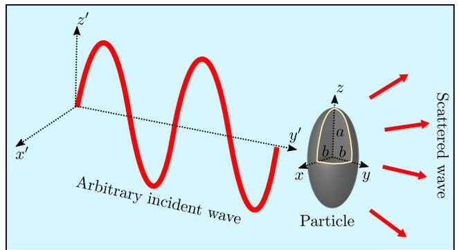
FIG. 1. The acoustic wave scattering by the spheroidal particle in a fluid medium. The particle has a major and minor semiaxis denoted by  $a$  and  $b$ . The arbitrary incoming beam is depicted as a red sinusoidal line. The scattered waves are represented by red arrows. The geometric center of the spheroid defines the particle frame of reference,  $\mathbf{r} = (x, y, z)$ . The laboratory frame of reference is the primed Cartesian axes.
