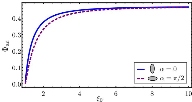
FIG. 5. The acoustophoretic factor  $\Phi_{ac}$  versus the geometric parameter  $\xi_0$  for different particle orientations.
