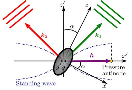
FIG. 3. Two plane waves crossing at right angle and interacting with a spheroidal particle in the  $x'z'$  plane. The particle frame corresponds to the  $x$  and  $z$  axes. The angle  $\alpha$  gives the particle orientation with respect to the  $z'$ -axis. The  $y'$ - and  $y$ -axis are going into the screen. The wavevectors  $\mathbf{k}_1$  and  $\mathbf{k}_2$  are depicted by red and green arrows. The vector  $\mathbf{h}$  (purple arrow) points to a transverse pressure antinode.
