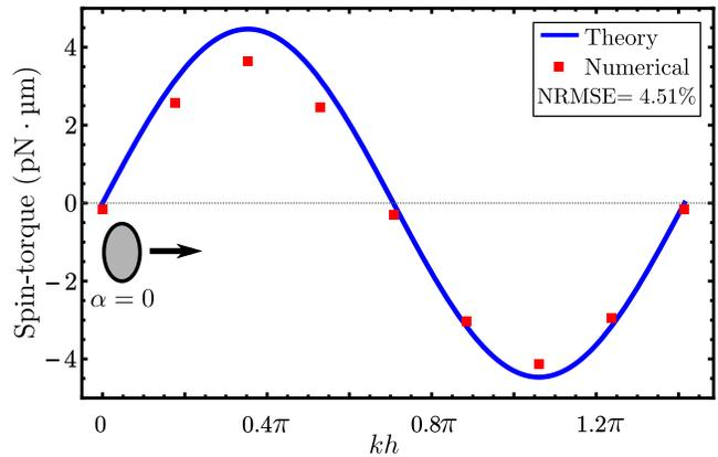
FIG. 11. The theoretical and numerical spin-torque on the spheroidal particle with a fixed orientation  $\alpha = 0$ . The particle (gray ellipse) has a geometric parameter of  $\xi_0 = 1.3181$  and its position varies from an antinode to a node. The simulational parameters are shown in Table I.
