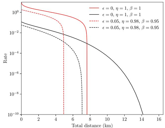
FIG. 4: Rates of the symmetric protocol function of the total distance between Alice and Bob with  $\sigma_A$  and  $\sigma_B$  optimized (black lines). For comparison, we include the original Gaussian MDI protocol with optimal parameters (red lines). The solid lines correspond to the pure-loss protocols with ideal parameters  $\eta = 1$  and  $\beta = 1$ , while the dashed lines correspond to a realistic scenario in which  $\epsilon = 0.05$ ,  $\eta = 0.98$  and  $\beta = 0.95$ .
