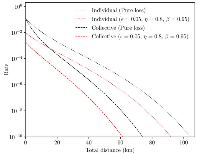
FIG. 6: Rates of the symmetric protocol with restricted eavesdropping as a function of the total distance between Alice and Bob with  $\sigma_A$  and  $\mu$  optimized. The black lines correspond to the pure-loss case with perfect detection and reconciliation while the red lines represent the rate with parameters  $\epsilon = 0.05$ ,  $\eta = 0.8$ , and  $\beta = 0.95$ .
