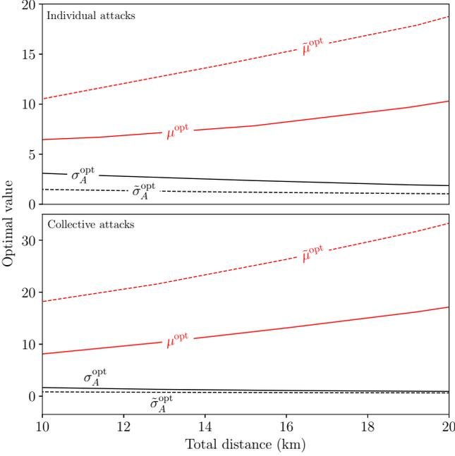
FIG. 7: Optimal values of  $\mu$  (red lines) and  $\sigma_A$  (black lines) for the symmetric protocol with restricted eavesdropping under individual (top panel) and collective (bottom panel) attacks. The solid lines represent the optimal parameters for the pure-loss case with ideal detection efficiency and the dashed lines represent the optimal values under parameters  $\epsilon = 0.05$ ,  $\eta = 0.8$  and  $\beta = 0.95$ .
