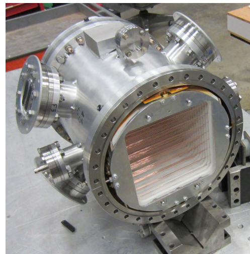
FIG. 4. Assembled target-detector chamber. The chamber consisted of an all aluminum cylindrical housing (except for the conflat flange knife edges, which were friction welded onto the aluminum), several signal, high voltage and gas feedthroughs, and the wire frame stack. The chamber windows (not shown here) consisted of 0.5 mm thick aluminum machined down from 12 inch aluminum blank conflat flanges. The chamber had an inner diameter of 254 mm and a length of 338 mm.
