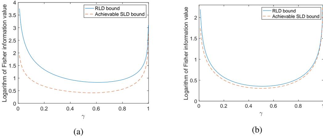
Figure 3: (a) Logarithm of RLD bound and achievable SLD bound versus loss  $\gamma$  for noise  $N = 0.2$ , when estimating the loss  $\gamma$ . (b) Logarithm of the RLD bound and achievable SLD bound versus loss  $\gamma$  for noise  $N = 0.45$ , when estimating the loss  $\gamma$ .
