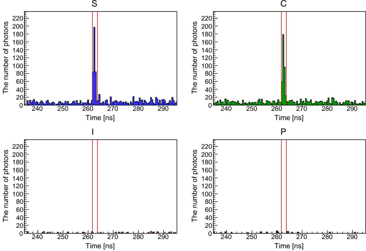
FIG. 7. Arrival time distributions of the number of observed photons in the case of the P-pol.(creation) + P-pol.(inducing) combination for individual trigger patterns at 10 Pa. Individual time windows in which signal photons are expected to be detected are indicated with the two red lines.
