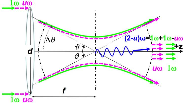
FIG. 1. A quasi-parallel collision system (QPS) combining two-color laser fields with beam diameter  $d$  and focal length  $f$ , where the incident angle  $\vartheta$  is subject to  $0 < \vartheta \leq \Delta\theta$ , which is unavoidable because of the ambiguity of the wave vectors of the incident photons due to the nature of the focused lasers. This figure is reproduced from [7] with a slight modification.
