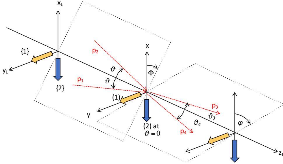
FIG. 2. Definitions of linear polarization directions and rotation angles in focused collision geometry. This figure is reproduced from [7] with a slight modification.
