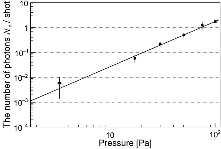
FIG. 8. Pressure dependence of the number of four-wave mixing photons per shot from the residual atoms inside the interaction chamber when the two beams with the same linear polarization directions, P-pol.(creation) + P-pol.(inducing), are focused.
