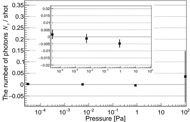
FIG. 10. Pressure independence of the number of four-wave mixing photons per shot from the residual atoms inside the interaction chamber when the two beams with the orthogonal linear polarization combination, P-pol.(creation) + S-pol.(inducing), are focused.
