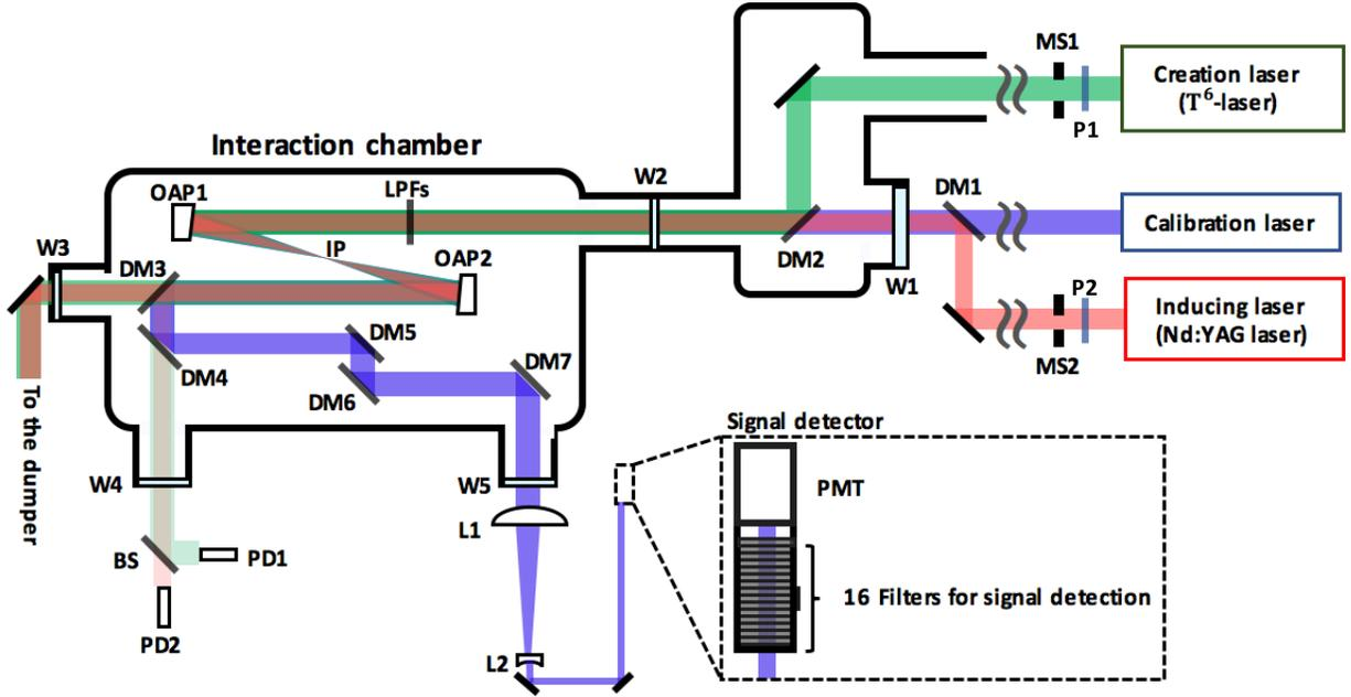
FIG. 3. Schematic of the searching system contained in a beam transport chamber and an interaction chamber designed to achieve  $10^{-8}$  Pa.
