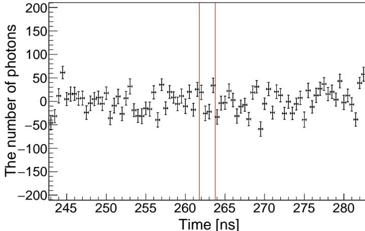
FIG. 12. Arrival time distribution of the number of photons obtained by applying Eq. (9) to the other timing windows including that of the four-wave mixing signal enclosed by the two red lines at  $3.7 \times 10^{-5}$  Pa in the case of the orthogonal polarization combination, P-pol.(creation) and S-pol.(inducing).
