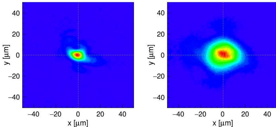
FIG. 4. Beam profiles of creation (left) and inducing (right) lasers at IP captured by a common CCD camera.
