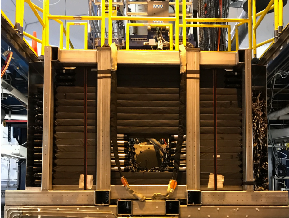
Figure 1: The backward angle neutron detector (BAND) installed in Hall B at Jefferson Lab.
