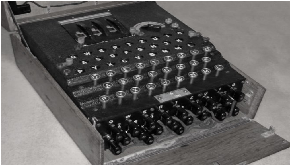
Figure 1: Exterior view of Enigma Showing front plugboard with cables 1
