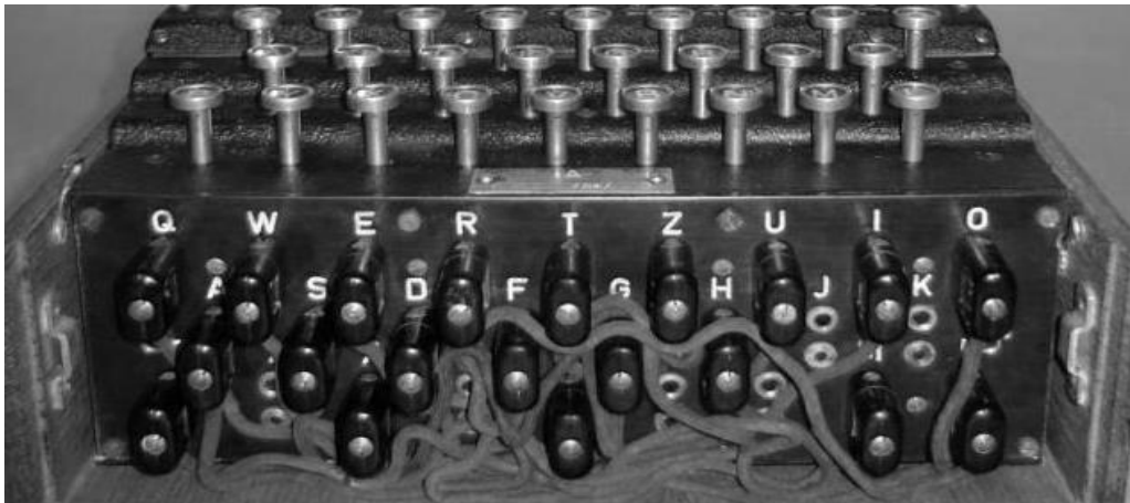
Figure 2: Close-up of Plugboard with cables 2
