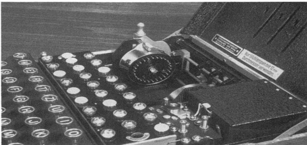
Figure 8: Reflector with rotors removed 9
