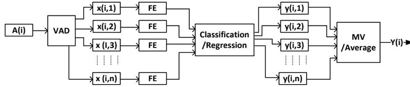
Figure 1: *System Architecture*:  $A(i)$ , the audio recording of  $i^{\text{th}}$  subjects is segmented using voice activity detection (VAD) into  $n$  segments  $x(i, n)$ . Feature extraction (FE) is performed at segment level. The output of classification or regression for the  $n^{\text{th}}$  segment of the  $i^{\text{th}}$  audio recording is denoted  $y(i, n)$ . MV outputs the majority voting for classification, and Average the mean regression score.
