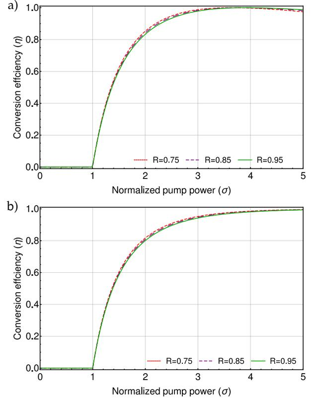
FIG. 3: DROPO: Conversion efficiency  $\eta$  as a function of pump power (normalized by the threshold power)  $\sigma$  for  $R_1 = \{75\%, 85\%, 95\%\}$ . Simulations with a) a  $\chi^{(2)}$  gain medium and b) a  $\chi^{(3)}$  gain medium.
