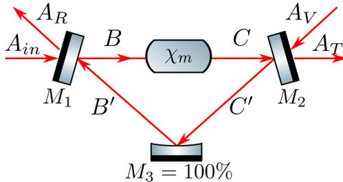
FIG. 6: Representation of the fields inside the cavity with a gain medium  $\chi^{(m)}$ .  $M_1$  and  $M_2$  are the input and output mirrors, with reflectivities (transmissivities) coefficients  $\mathbf{R}$  ( $\mathbf{T}$ ) and  $\mathbf{R}'$  ( $\mathbf{T}'$ ).
