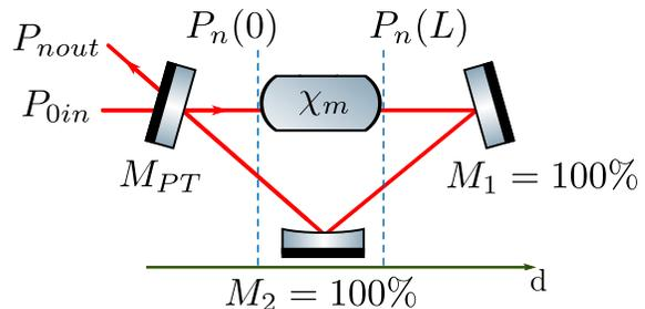
FIG. 1: OPO model using a ring cavity with two highly reflective mirrors ( $M_1 = M_2 = 1$ ), an output coupler  $M_{PT}$  and a gain medium with length  $L$ . The  $M_{PT}$  reflectance coefficient for the pump beam is  $R_0$  and for both, signal and idler beams,  $R_1$ .
