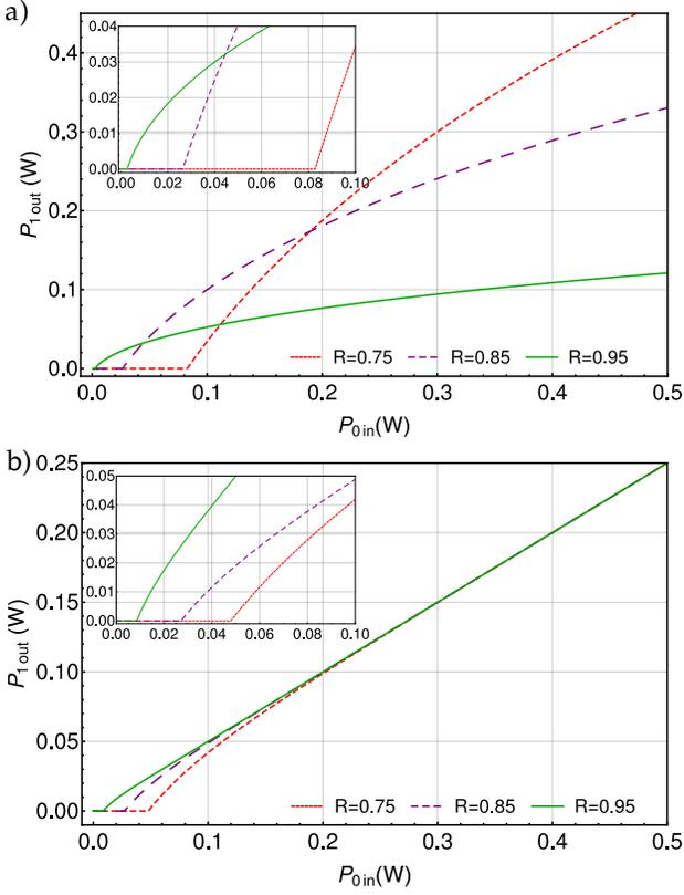
FIG. 2: DROPO:  $P_{out}$  as a function of  $P_{in}$  for different reflectivity coefficients  $R_1 = \{75\%, 85\%, 95\%\}$ . Simulations considering (a) a  $\chi^{(2)}$  gain medium with  $\kappa^{(2)} = 0.5W^{-1/2}$  and in (b) a  $\chi^{(3)}$  gain medium with  $\kappa^{(3)} = 3W^{-1}$ .
