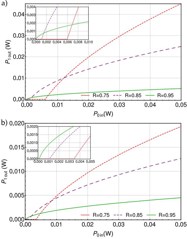
FIG. 4: TROPO:  $P_{1out}$  in function of  $P_{0in}$  for different reflectivity coefficients  $R_1 = \{75\%, 85\%, 95\%\}$ . Simulations considering a) a  $\chi^{(2)}$  gain medium and in b) a  $\chi^{(3)}$  gain medium.
