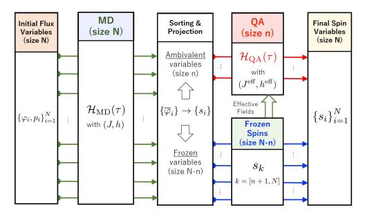
Figure 5: Flowchart of the Hybrid Quantum Annealing (HQA) via Molecular Dynamics (MD).
