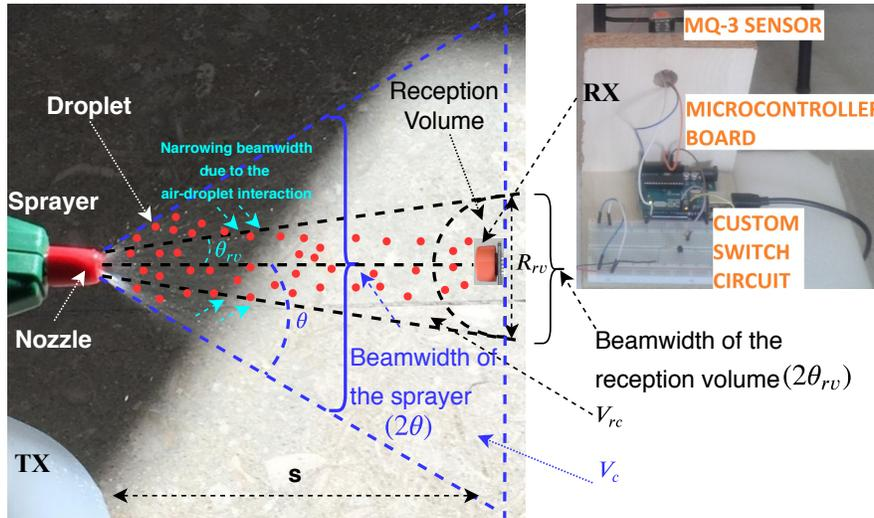
Fig. 1: The experimental setup and parameters.
