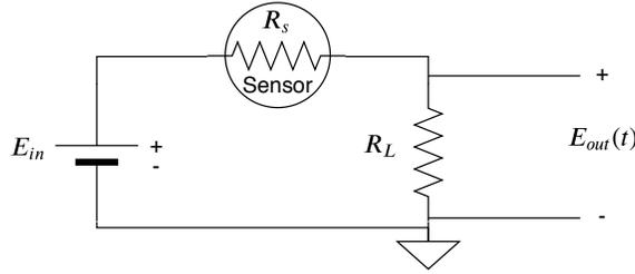
Fig. 4: Sensor Measurement Circuit.
