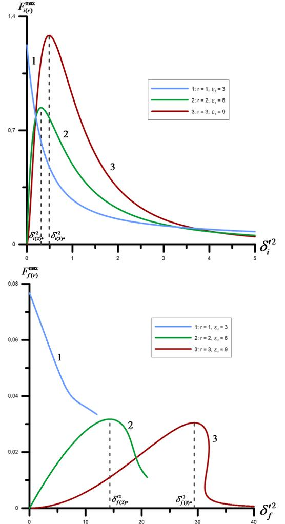
FIG. 6. The dependencies of the functions  $F_{i(r)}^{max}$  (for the channel A) and  $F_{f(r)}^{max}$  (for the channel B) (120) on the corresponding parameters  $\delta_i'^2$  and  $\delta_f'^2$  for the first, second and third resonances. The characteristic parameter is  $\varepsilon_1 = 3$  (the characteristic energy is  $E_1 = 41.7 GeV$ , the energy of the initial electron is  $E_i = 125.1 GeV$ ).
