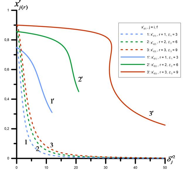
FIG. 3. The dependency of the resonant frequency of a spontaneous photon on the radiation angle. The dashed lines delineate the first three resonant frequencies of the channel A (43) ( $j = i$ ), the solid lines illustrate the first three resonant frequencies of the channel B (52), (48) ( $j = f$ ). The characteristic parameter  $\varepsilon_1 = 3$  (the characteristic energy is  $E_1 = 41.7 \text{ GeV}$ , the energy of the initial electron is  $E_i = 125.1 \text{ GeV}$ ).
