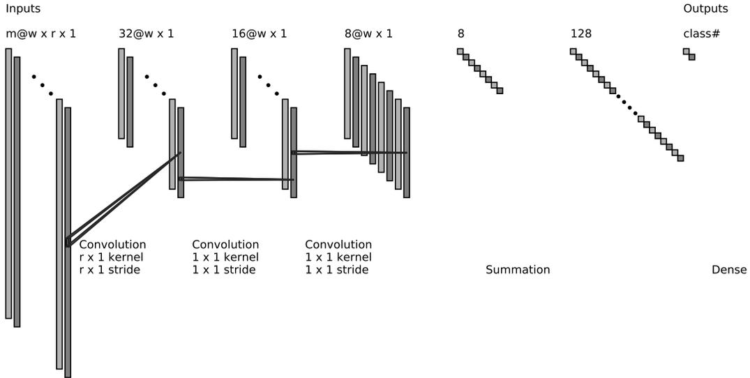
Fig. 4: Convolutional architecture. In the first layer,  $m$  is the dimension of the vertex feature map,  $w$  is the maximum number of vertices in a set of graphs, and  $r$  is the size of the receptive field.
