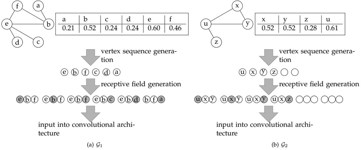
Fig. 3: Illustration of the generation of vertex sequences and the corresponding receptive fields for undirected graphs  $\mathcal{G}_1$  and  $\mathcal{G}_2$ . The two tables beside graphs  $\mathcal{G}_1$  and  $\mathcal{G}_2$  contain the eigenvector centrality value of each vertex.
