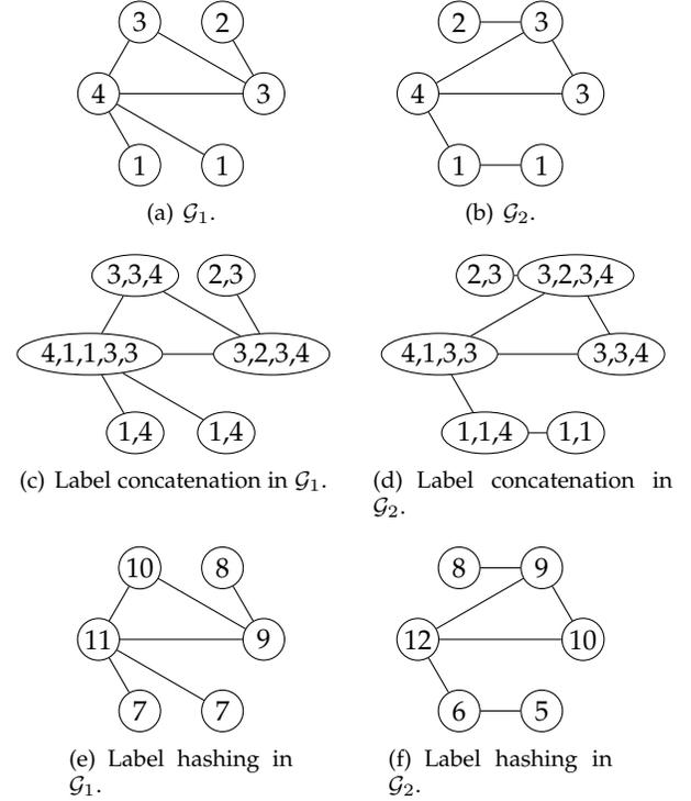
Fig. 2: Illustration of one iteration of the WL test of graph isomorphism algorithm for graphs. For subfigures (a) and (b),  $\Sigma = \{1, 2, 3, 4\}$ . For subfigures (e) and (f),  $\Sigma = \{5, 6, 7, 8, 9, 10, 11, 12\}$
