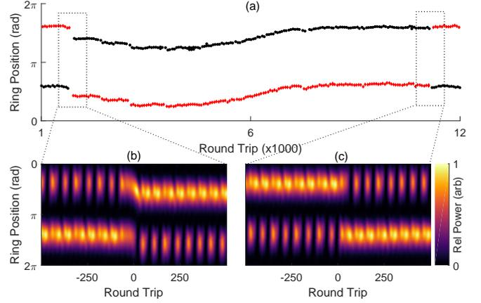
FIG. 13. *Spontaneous Spatial Shifts* (a) All peaks detected for a spontaneous spatial shifting behavior. Red dots indicate the short peaks which oscillate between a normalized magnitude of 0.7 and 0, while black dots show the high peaks which oscillate between 0.7 and 1. (b) Two shifting events when the relative location of the two stable modulating solitons abruptly shifts within the ring.
