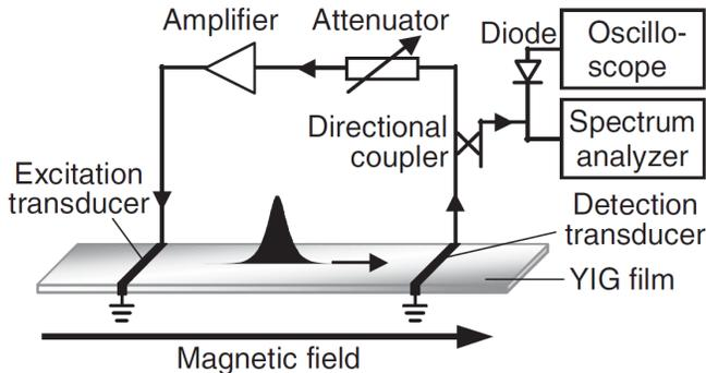
FIG. 1. *Diagram of an active magnetic thin film-based feedback ring.* A spin wave feedback ring constructed of a nonlinear, dispersive waveguide (the YIG film) coupled to an electronic feedback loop via two transducers. The ring has a linear, fixed amplifier and a variable attenuator. Observation equipment is attached via a directional coupler. Reprinted with permission [10].
