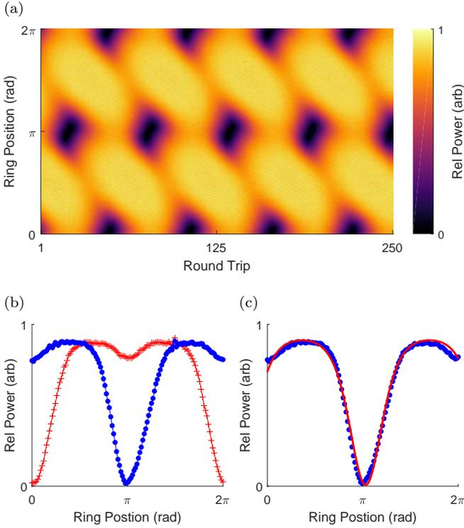
FIG. 7. *Dark solitary wave periodic breathing.* A single dark solitary wave breathing at a fixed frequency from the center of the feedback ring to the edge. (a) A spatiotemporal plot of the spin wave power. (b) A single round trip of the dark solitary wave in the center of the ring (dotted blue) and at the edge of the ring a half breath later (crossed red). (c) A fit of a single central round trip to the generalized dark solitary Jacobi-elliptic solution to the NLS.
