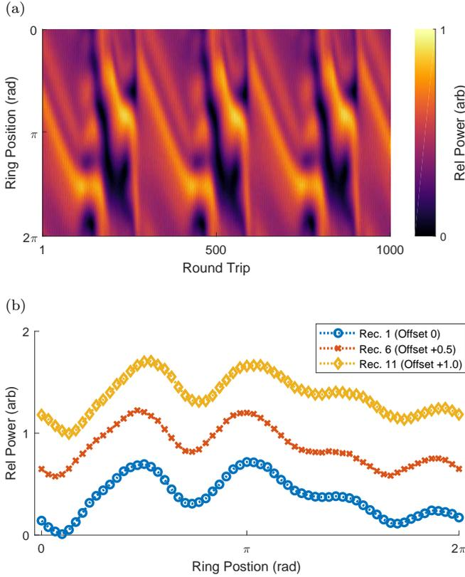
FIG. 12. *Bright solitary wave recurrence.* (a) Four bright solitary waves undergoing a complex recurrence. Format is the same as figure 11. The nontrivial repeating shape can be identified easily, as can its periodicity. (b) The single round trips of recurrence 1, 11 and 16. These plots have been shifted by 0, 0.5 and 1 in power, respectively, to aid with direct comparison.
