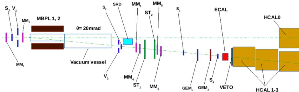
Рис. 4: Schematic illustration of the setup to search for invisible decays of the bremsstrahlung  $A'$ s produced in the reaction  $eZ \rightarrow eZA'$  of 100 GeV  $e^-$  incident on the active ECAL target.
