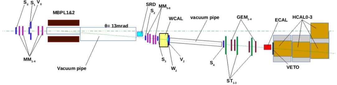
Рис. 5: Schematic illustration of the setup to search for visible  $A', X \rightarrow e^+e^-$  decays of the bremsstrahlung  $A', X$  produced in the reaction  $eZ \rightarrow eZA'$  of 100 GeV  $e^-$  incident on the active WCAL target.
