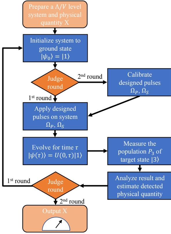
Figure 1. Flowchart for the quantum sensing in three level system.  $X$  is a unknown physical quantity to be measured.
