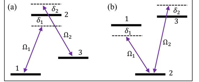
Figure 2. Schematic of generic three-level system. (a)  $\Lambda$  type level structure with detuning. (b)  $V$  type level structure with detuning.
