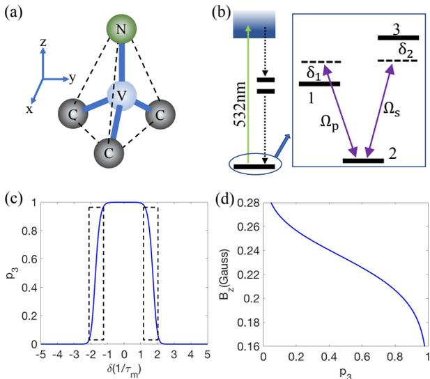
Figure 5. Schematic of solid spin for detecting magnetic field. (a) The structure of an NV color centres in diamond. (b) Level structure of NV centre in diamond. The levels in the right rectangle are triplet structure in ground state. (c) The curve for population vs detuning with duration  $\tau = 10\tau_m$ . (d) The magnetometer in the domain labelled with dashed rectangle in (c).
