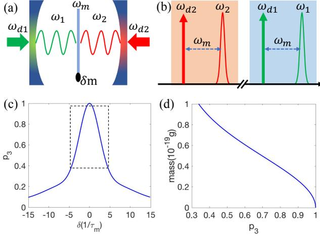
Figure 4. Schematic of same color optomechanical mass sensor. (a) Generic setup for optomechanical system. Two optical cavities couple to each other by driving a mechanical oscillator. The small dot represents a deposited mass on the mechanical oscillator. (b) Red detuning drivings for two optomechanical interactions. (c) The curve for population vs detuning with duration  $\tau = 1.0\tau_m$ . (d) The mass sensor in the domain labelled with dashed rectangle in (c).
