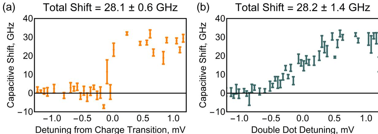
**FIG. 13:** Capacitive shift experienced by the right double dot due to a transition in the left double dot from (a) the (1,0) to the (1,1) charge state and (b) the (1,0) to the (0,1) charge state. Note that the abrupt transition in (a) is because the charge transition being swept is a cotunneling process with a very slow tunnel rate [15].
