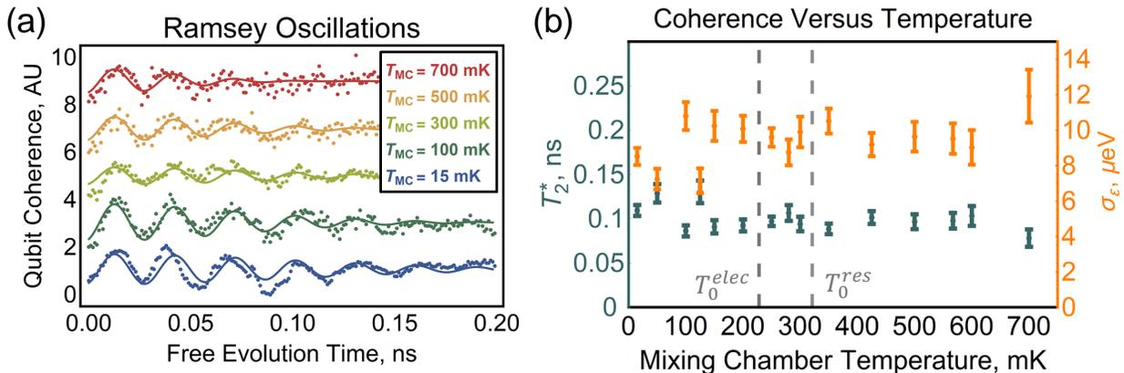
**FIG. 10:** (a) Ramsey data measured on the right double dot as a function of temperature. These linecuts were taken at  $\epsilon/h = -33$  GHz. (b) Inhomogeneous dephasing time and quasistatic charge noise extracted from the temperature-dependent Ramsey data.
