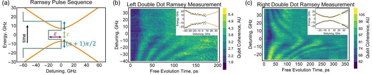
**FIG. 2:** (a) Dispersion and pulse sequence for measuring Ramsey oscillations at a detuning  $\varepsilon$  for a free evolution time  $\tau$ . (b,c) Ramsey oscillations measured in the (b) left and (c) right double dots. The extracted charge qubit dispersions with (b)  $t_c^L/h = 9.2$  GHz and (c)  $t_c^R/h = 5.0$  GHz are shown in the insets.
