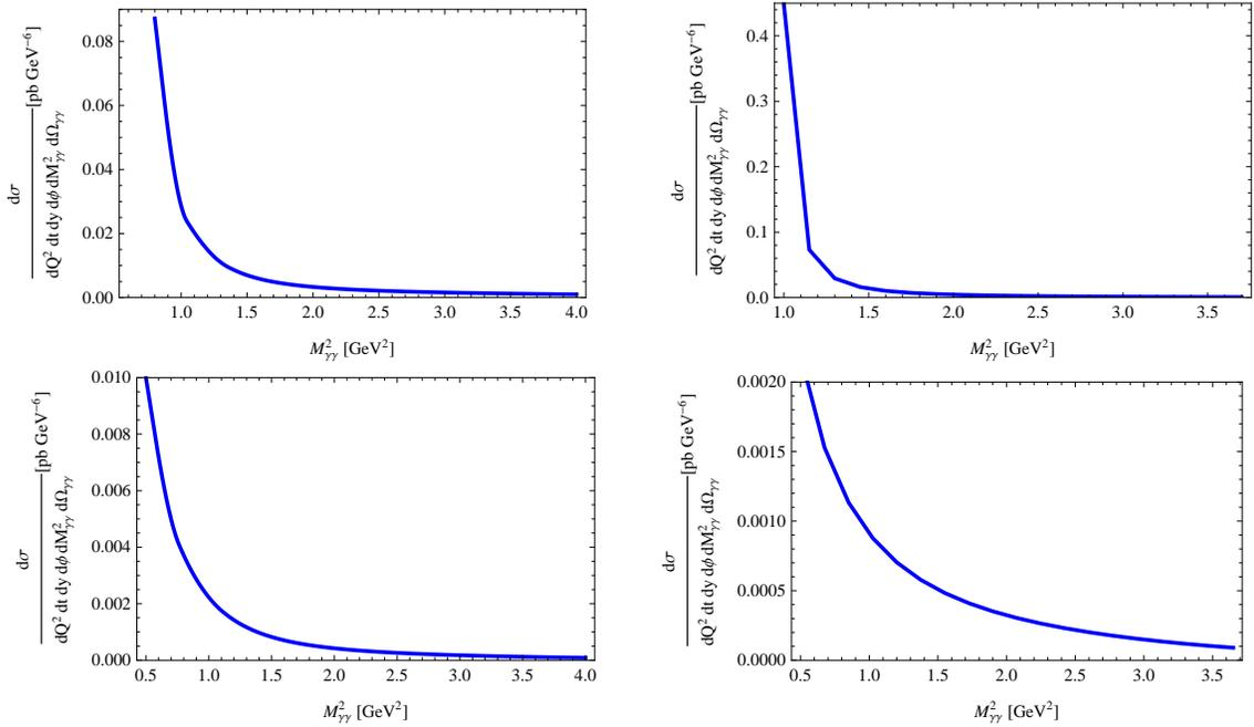
FIG. 9:  $M_{\gamma\gamma}^2$  dependence of the contribution of the double Bethe-Heitler process to the differential cross-section at  $\theta = 3\pi/8$ ,  $y = 0.8$ , for  $\phi_{\gamma\gamma} = 0$  (first line) or  $\phi_{\gamma\gamma} = \pi/2$  (second line), and for  $Q^2 = 1$  (resp. 2)  $\text{GeV}^2$  on the left (resp. right) panel.
