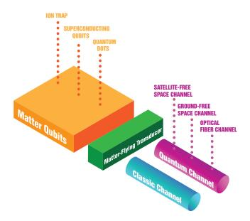
Fig. 5. Pictorial representation of a matter-flying transducer, which is needed to convert matter qubits – i.e., qubits for information processing/storing – into flying qubits – i.e., qubits for information transmission – and vice versa.
