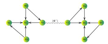
Fig. 7. Coupling map representing physical architecture of two quantum devices **ibmqx2** interconnected via the quantum teleportation paradigm. Nodes labeled with  $c_0$  and  $c_1$  denote *communication qubits*, and the dotted line indicates that they are in the entangled state  $|\Phi^+\rangle$ , i.e., they form an EPR pair. Conversely,  $q_i$  with  $i \in \{0, 1, 2, 3\}$  denote *data qubits* – i.e., qubits available for computing tasks.
