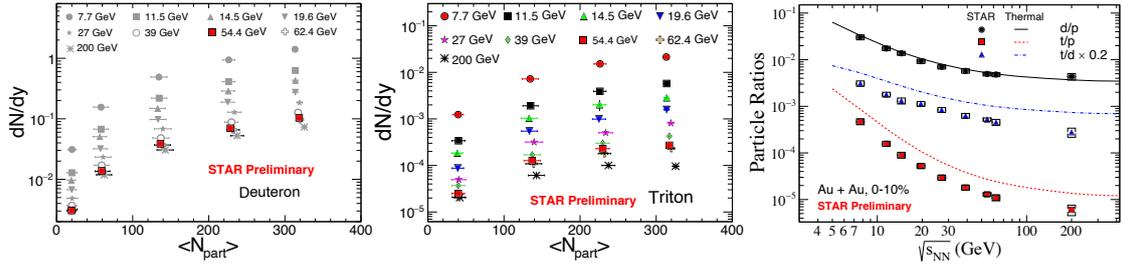
Fig. 3. Centrality dependence of  $dN/dy$  of  $d$  (left panel) and  $t$  (middle panel) in Au+Au collisions. Energy dependence of  $d/p$ ,  $t/p$ , and  $t/d$  (right panel) ratios for 0-10% central Au+Au collisions at BES-I energies. The dotted lines are thermal model predictions. The errors represent combined systematic and statistical uncertainties.
