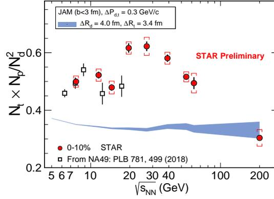
Fig. 4. Energy dependence of the light nuclei yield ratio  $N(t) \times N(p) / N^2(d)$  in central (0 – 10%) heavy-ion collisions. The red solid circles are the results measured in central (0–10%) Au+Au collisions at BES energies by the STAR experiment and the open squares are the results calculated from the Pb+Pb data of NA49 experiment [4]. The blue band represents the results of central Au+Au collisions ( $b < 3$  fm) from the JAM model calculations [10].
