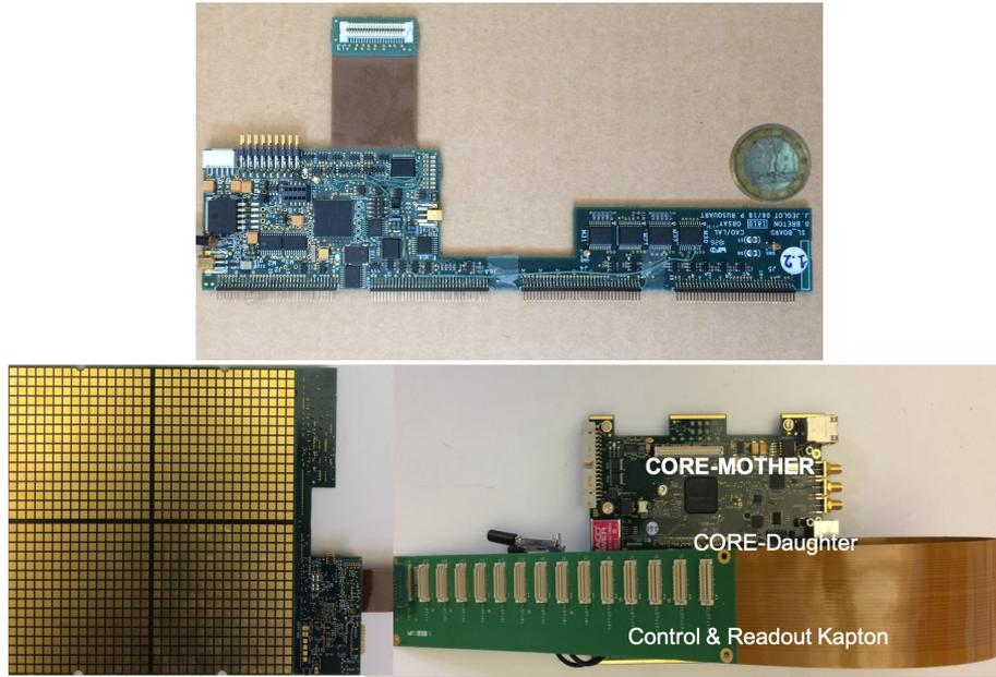
**Figure 2:** *Top: SL-Board for the digital readout and the power supply of the SiW ECAL layers. Bottom: Ensemble of ASU, control and readout kapton and control unit (CORE Mother + CORE Daughter). For details see text.*
