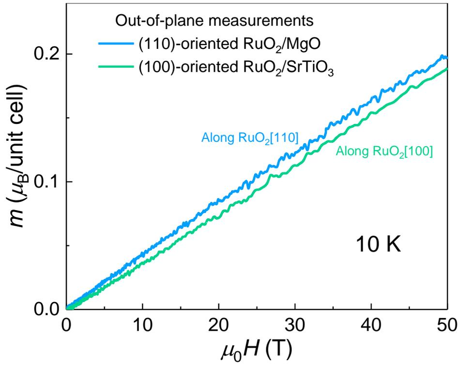
Supplementary Figure 6 | Out-of-plane magnetic moments of RuO<sub>2</sub> thin films obtained by pulsed-field measurements at 10 K.
