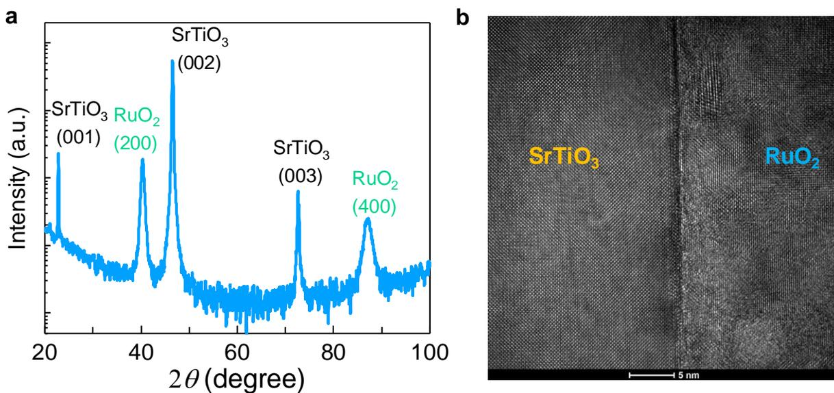
**Supplementary Figure 5 | Structural characterization** of a RuO<sub>2</sub>/SrTiO<sub>3</sub> heterostructure fabricated at 550°C and 10<sup>-3</sup> Torr oxygen partial pressure. **a.** X-ray diffraction pattern. **b.** Cross-section transmission electron microscopy image.
