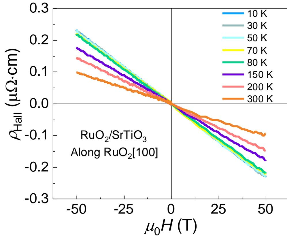
Supplementary Figure 8 | Total Hall signal of the (100)-oriented RuO<sub>2</sub>/SrTiO<sub>3</sub> film measured at various temperatures.
