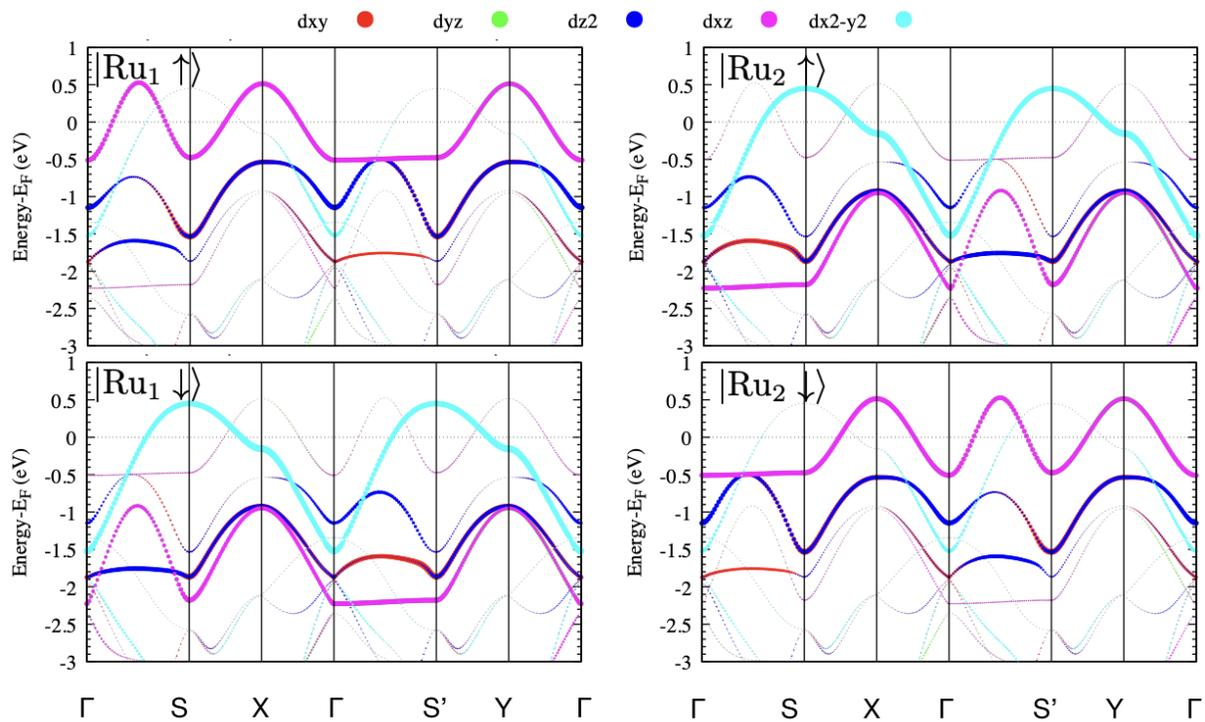
**Supplementary Figure 1** | Orbital (Ru  $d$ -states) and spin resolved energy bands in antiferromagnetic state calculated without spin-orbit interaction in VASP.
