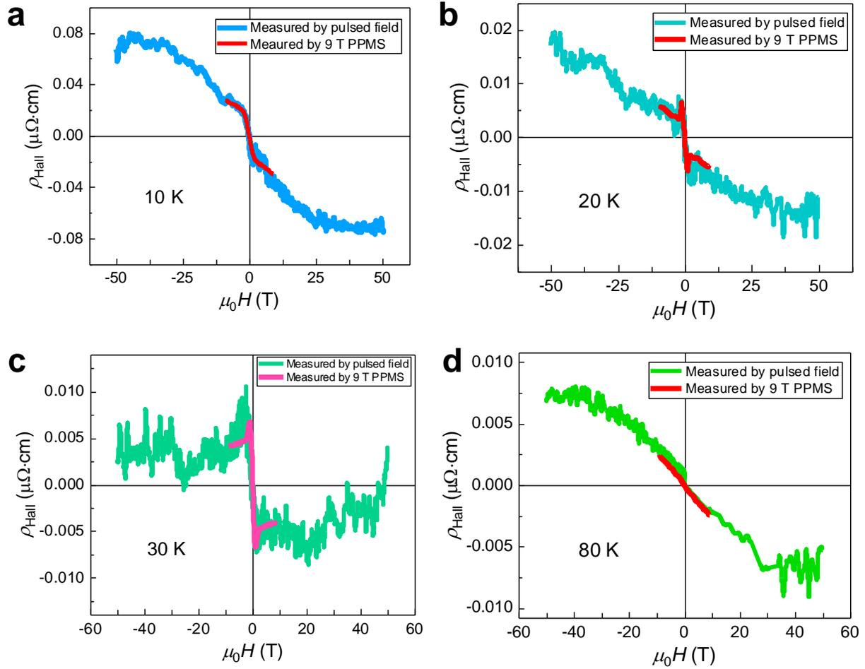
**Supplementary Figure 10 | Crystal Hall effect up to 50 T along the out-of-plane direction of the (110)-oriented RuO<sub>2</sub>/PMN-PT heterostructure obtained by pulsed-field and 9 T-PPMS measurements at different temperatures.**
