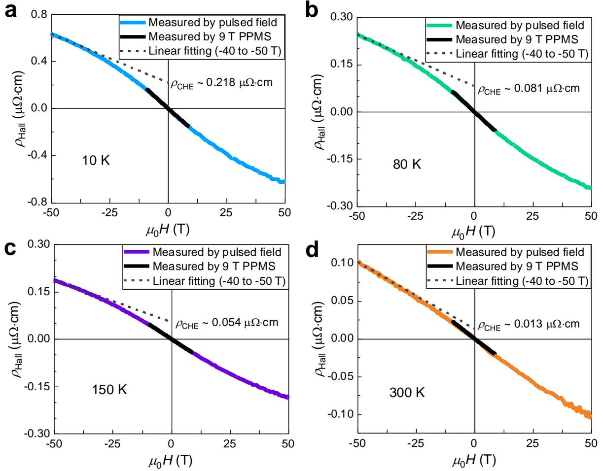
**Supplementary Figure 7 | Total Hall signal** for the RuO<sub>2</sub>/MgO film obtained by pulsed-field and static-field measurements at different temperatures. Dashed lines represent the linear fitting curves of the total Hall data between -40 and -50 T and the extrapolated zero-field Hall resistivity values are used to represent the zero-field crystal Hall resistivities.
