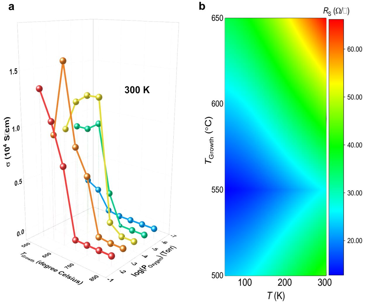
**Supplementary Figure 4 | Conductivity optimization and characterization of RuO<sub>2</sub> thin films on MgO (ref. <sup>S3</sup>).** **a.** Phase diagram of electrical conductivity of RuO<sub>2</sub> thin films fabricated by pulsed laser deposition at different oxygen pressures and deposition temperatures. **b.** Temperature-dependent sheet resistance contour mapping of the RuO<sub>2</sub> films fabricated in the growth temperature range between 500 and 650 °C.
