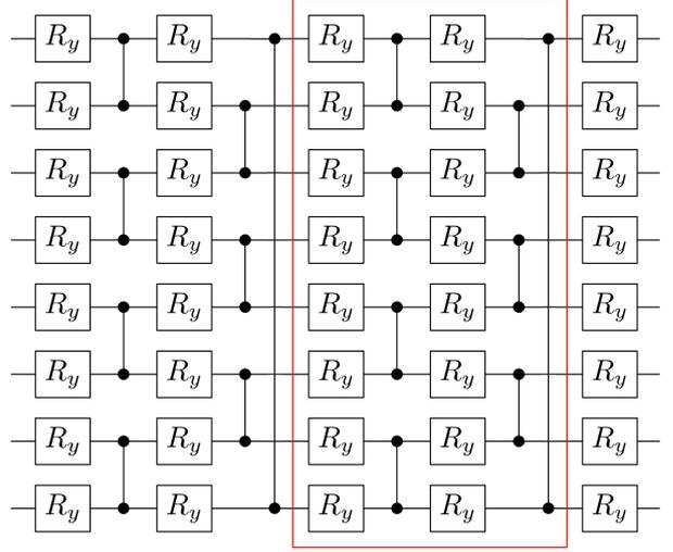
Figure 1: Variational quantum ansatz for  $\tilde{U}(\vec{\theta})$  employed in our simulations. As indicated by the red box, each layer is composed of  $CZ$  gates acting on alternating pairs of neighboring qubits which are preceded by  $R_y(\theta_i)$  qubit rotations,  $R_y(\theta_i) = e^{-i\theta_i Y/2}$ . After implementing the layered ansatz, a final layer of  $R_y(\theta_i)$  qubit gates is applied. Here, it is shown the case of two layers and  $n = 8$  qubits.
