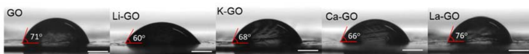
Supplementary Fig. 2 | Contact angle of cation modified graphene oxide (GO) membranes. Water contact angle of pristine GO and Li, K, Ca, and La modified GO membranes. Scale bar, 750 \mu\text{m} .
