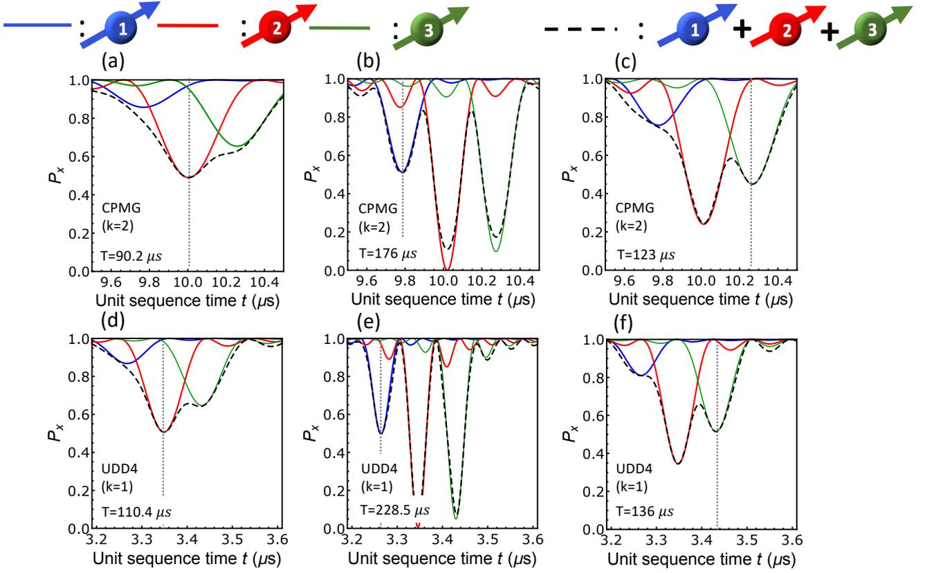
FIG. 15. Comparison of UDD4 and CPMG for the case of three nuclear spins. Like in Fig. 4, here we plot the probability  $P_x$  of preserving the electrons initial  $|x\rangle$  state after the (a,b,c) CPMG protocol and the (d,e,f) UDD4 protocol.
