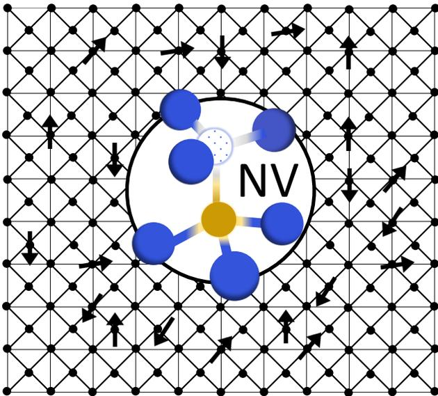
FIG. 1. Sketch of an NV center in diamond (top view of an extended (100) plane). The defect consists of a nitrogen substitute (yellow) and a vacancy (dotted white) at the neighboring site, and features a localized  $S = 1$  electronic spin. Individual nuclear spins (black arrows) are coupled via dipolar hyperfine interaction to the NV electronic spin.
