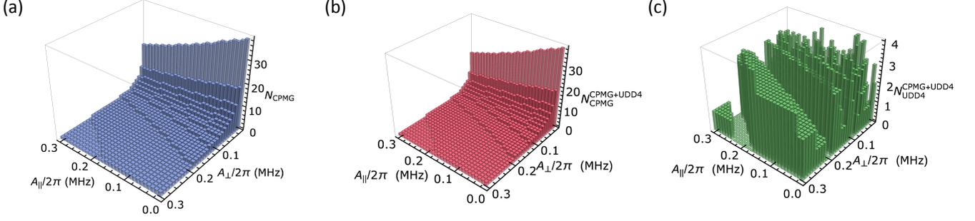
FIG. 13. (a) Integer values for the iteration number  $N_{\text{CPMG}}$  used in the fidelity plot of Figs. 7(c). (b,c) Integer values for the iteration numbers  $N_{\text{CPMG+UDD4}}^{\text{CPMG}}$  and  $N_{\text{UDD4}}^{\text{CPMG+UDD4}}$  used in the fidelity plots of Fig. 7(d). The Larmor frequency is set equal to  $\omega_L/2\pi = 0.5$  MHz.
