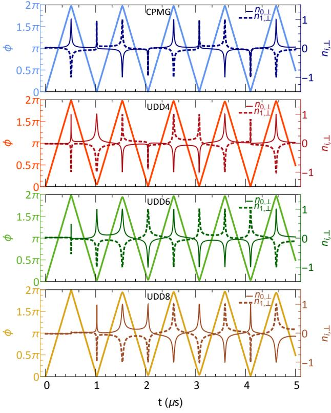
FIG. 11. Rotation angle  $\phi$  and perpendicular components of the unit axes,  $n_{0,\perp}$  and  $n_{1,\perp}$ , vs the unit sequence time  $t$  for different UDD $n$  sequences with even  $n$ . The values for the system parameters used to make the plots are  $\omega_L/2\pi = 2$  MHz and  $A_{\parallel}/2\pi = A_{\perp}/2\pi = 0.1$  MHz. Note that whenever a peak(dip) of  $n_{0,\perp}$  coincides with the dip(peak) of  $n_{1,\perp}$  the nuclear spin undergoes a conditional rotation.
