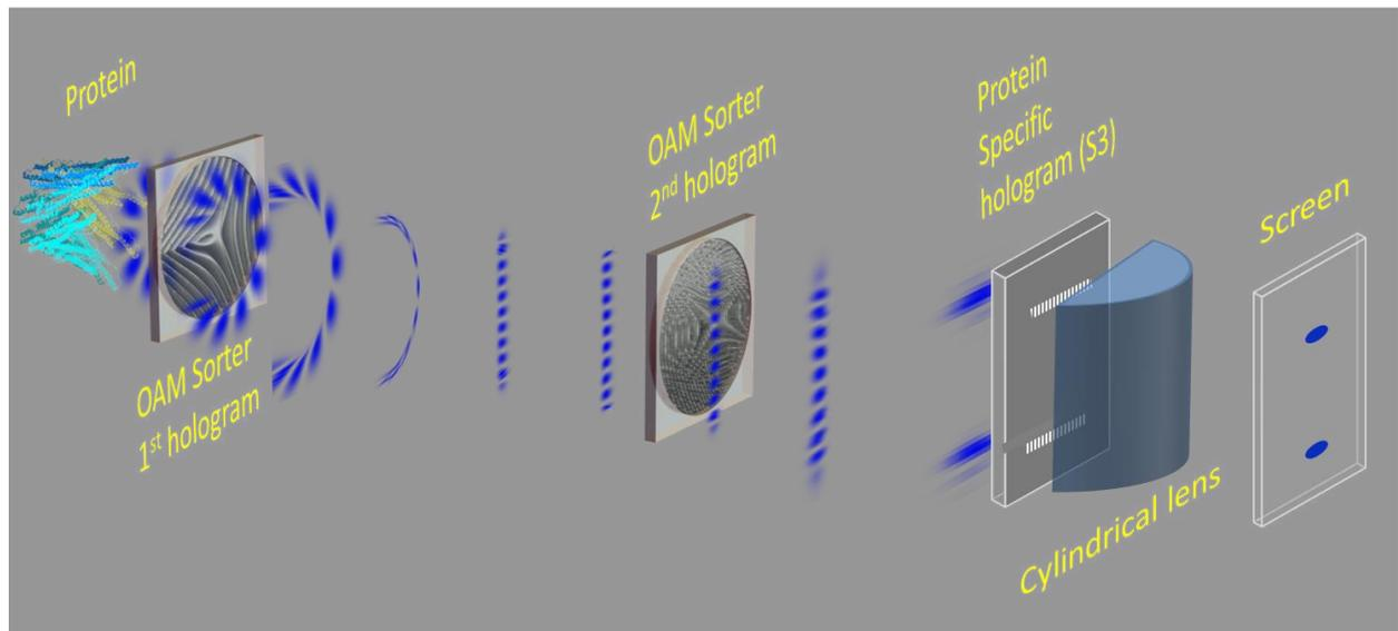
**Fig 1.** Schematic view of the generalized OAM sorter. With respect to the standard OAM sorter, a third phase element is added. The structure of such third element is adapted to the radial structure of the proteins to be recognized.
