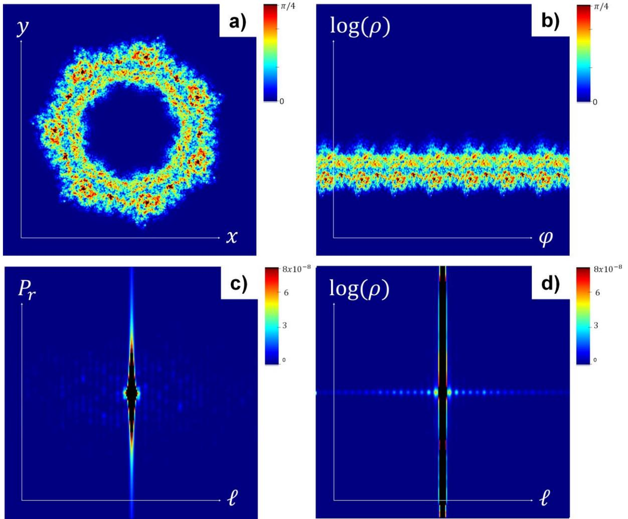
**Fig 2.** Series of unitary transformation that the different electrostatic elements apply to the electron wave function in the case of the protein Pa. In particular, we show: the phase modulation of the electron wave function in (a) Cartesian and (b) log-polar coordinates; (c) the intensity of the diffraction to the OAM sorter in (c) the radial momentum space and (d) after optimal radial sorting.
