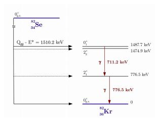
Figure 1: Decay scheme of the <sup>82</sup>Se  $\beta\beta$  decay to the  $0^+_1$  excited state with the emission of two electrons sharing 1510.2 keV and two prompt  $\gamma$ -rays with energies of 711.2 and 776.5 keV [36].
