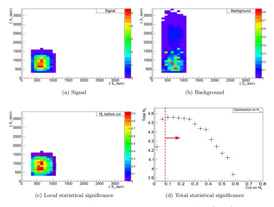
Figure 10: Total electron energy vs total  $\gamma$ -rays energy distributions for  $2\nu\beta\beta(0_{gs}^+ \to 0_1^+)$  signal simulation (10(a)) and background (10(b)). Local statistical significance distributions for each bin of this histogram (10(c)) with optimisation cut (dotted red line) on total statistical significance  $N_{\sigma}$  presented in Figure 10(d).
