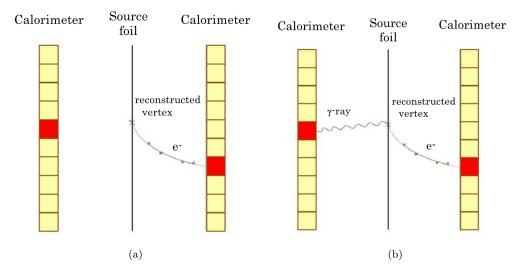
Figure 5: Event sketch with track reconstruction (5(a)) and scintillator association (5(b)). The reconstruction defines a  $\gamma$ -ray as energy deposit in a scintillator without any associated track. It can link it to the vertex in Figure 5(b).
