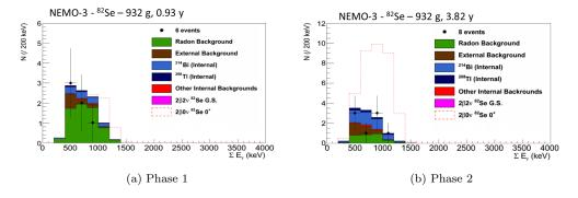
Figure 15: Total  $\gamma$ -rays energy distributions after selection for the  $0\nu\beta\beta$   $(0_{gs}^+ \rightarrow 0_1^+)$  transition, for Phase 1 in Figure 15(a) and Phase 2 in Figure 15(b). Experimental data events are compared to the MC simulation for the different backgrounds. The dotted red line represents the simulated signal with a half-life of  $3 \times 10^{21}$  years.
