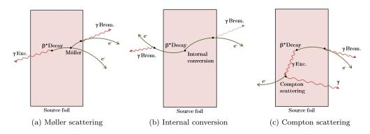
Figure 3: Mechanisms producing  $2e2\gamma$  events from internal contamination of  $\beta$  emitters inside the source foils.  $\beta$ -decay to excited state followed by Møller scattering and bremsstrahlung (3(a)),  $\beta$ -decay to excited state with internal conversion and double bremsstrahlung (3(b)),  $\beta$ -decay to excited state followed by Compton scattering and bremsstrahlung (3(c)).
