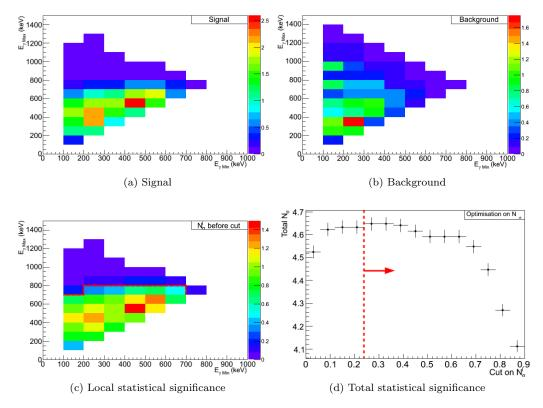
Figure 11:  $\gamma$ -ray 1 energy vs  $\gamma$ -ray 2 energy distributions for  $2\nu\beta\beta$   $(0_{gs}^+ \to 0_1^+)$  signal simulation (11(a)) and background (11(b)). Local statistical significance distributions for each bin of this histogram (11(c)) with optimisation cut (dotted red line) on total statistical significance  $N_{\sigma}$  presented in Figure 11(d).
