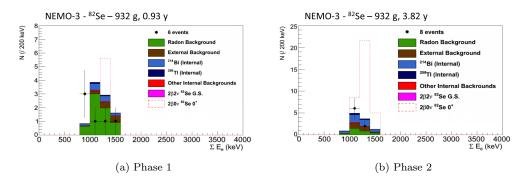
Figure 14: Total electron energy distributions after selection for the  $0\nu\beta\beta$   $(0_{gs}^+ \rightarrow 0_1^+)$  transition, for Phase 1 in Figure 14(a) and Phase 2 in Figure 14(b). Experimental data events are compared to the MC simulation for the different backgrounds. The dotted red line represents the simulated signal with a half-life of  $3 \times 10^{21}$  years.
