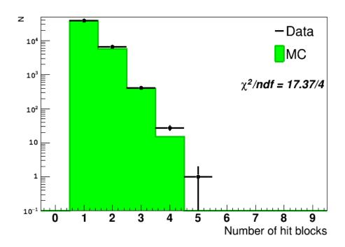
Figure 7: Number of scintillator blocks hit by a single  $\gamma$ -ray according to the path reconstruction calculated with the gamma tracking method, logarithmic scale. Data were acquired using  $\gamma$ -rays from the  $^{232}$ U radioactive sources and are compared to Monte-Carlo simulations.
