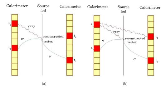
Figure 6: Example of an event reconstruction without using gamma tracking (6(a)). Only one of the two scintillators not associated to a track is consistent with the *internal* hypothesis, the other is neither *internal* nor *external*. The same event is reconstructed with gamma tracking (6(b)), the second scintillator can be associated to the first one under the assumption of Compton scattering.
