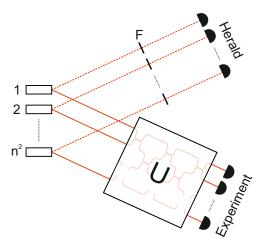
FIG. 1. A n-photon scattershot boson-sampling experiment has  $n^2$  heralded single-photon sources. Each source can send a photon to one of the input modes of the interferometer U. The other photon (dashed) is filtered (F) and is used as a herald.
