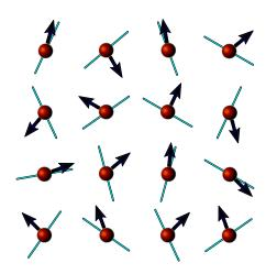
FIG. 1. Sketch plot of the two-dimensional RAM. Red discs depict sites of the lattice with spins (black arrows) on them. Random local anisotropy axis direction on each site is shown by light blue line.
