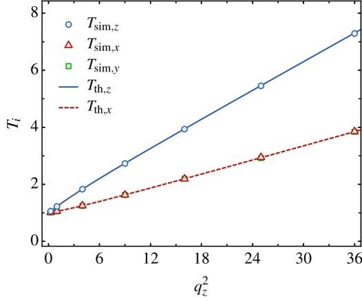
Figure 5. Comparison of the simulation results for  $T_i = \langle p_i^2 \rangle_{t \rightarrow \infty}$  ( $i = x, y, z$ ) with the analytical predictions (35) and (36) for an isotropic potential (21) with  $\alpha = 1$  for different kick strengths  $q_z$  along the  $z$ -direction. Note that the predicted  $\langle p_x^2 \rangle_\infty$  and  $\langle p_y^2 \rangle_\infty$  are identical.
