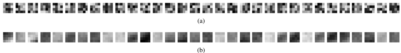
Fig. 19. Weights of the first convolutional layer. The size of each convolutional kernel is 4 \times 4 . Each kernel of 32 kernels in the first convolutional layer is shown in the forms of a tiny image. (a) Randomly initialized weights of the first convolution layer on the Salinas data set. (b) Learned weights of the first convolution layer on the Salinas data set.
