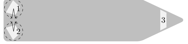
Fig. 2. Thruster configuration for vessel, where 1 and 2 are azimuth thrusters, and 3 is a tunnel thruster.
