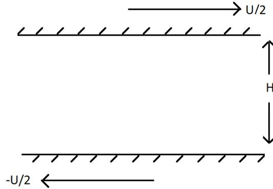
Figure 7: A representative sketch of the Couette flow setup. Two walls with a separation  $H$  are sheared in the opposite directions with velocity  $U/2$ .
