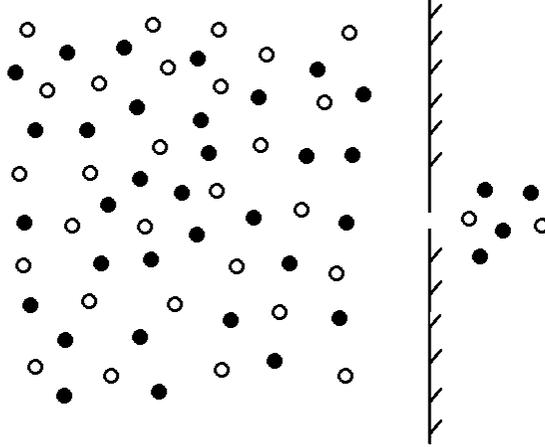
Figure 5: The lighter particles (in this case filled) escape through the hole faster than the heavier particles, with a factor proportional to the square root of their mass ratios.
