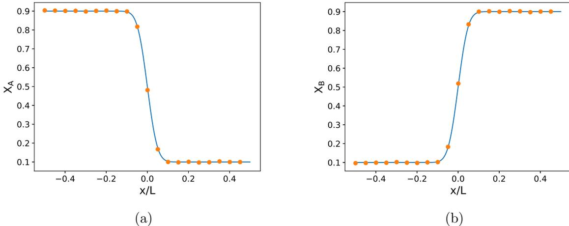
Figure 8: Plot of the concentrations after 20,000 time steps of the component a) A and b) B, in comparison with the analytical solution given by Eq.(89).
