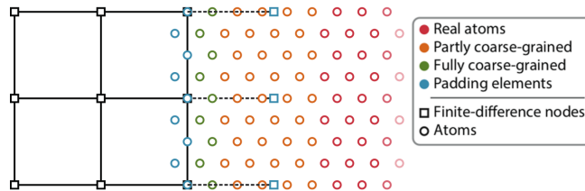
FIG. 1: Schematic representation of the atomistic-continuum interface. The fully atomistic region is represented by real atoms while the fully micromagnetic region is represented by finite-difference nodes. In the interface, both regions mix each other.
