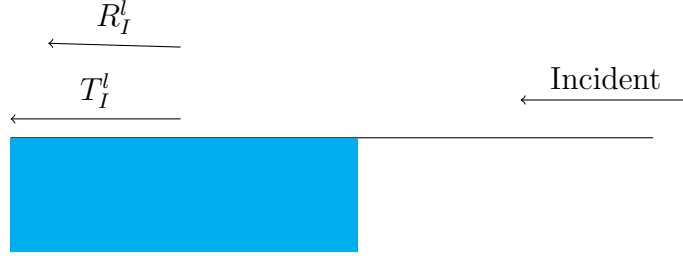
FIG. 15: Illustration of a plane wave incident onto the negative step function potential from the right. As this is in the interior of the BH both the transmitted and reflected portions of the mode are forced to travel further into the BH.
