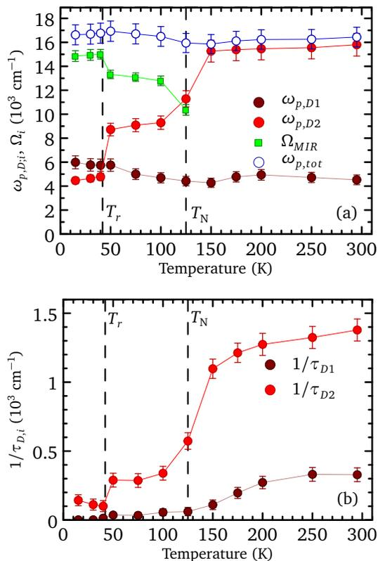
Figure 4. (a) The temperature dependence of the plasma frequencies of the narrow (D1) and broad (D2) Drude components, the oscillator strength of the mid-infrared peak ( $\Omega_{MIR}$ ), and the total when these three components are added in quadrature ( $\omega_{p,tot}$ ), for Sr<sub>0.67</sub>Na<sub>0.33</sub>Fe<sub>2</sub>As<sub>2</sub>. (b) The temperature dependence of the scattering rates of the narrow and broad Drude components.
