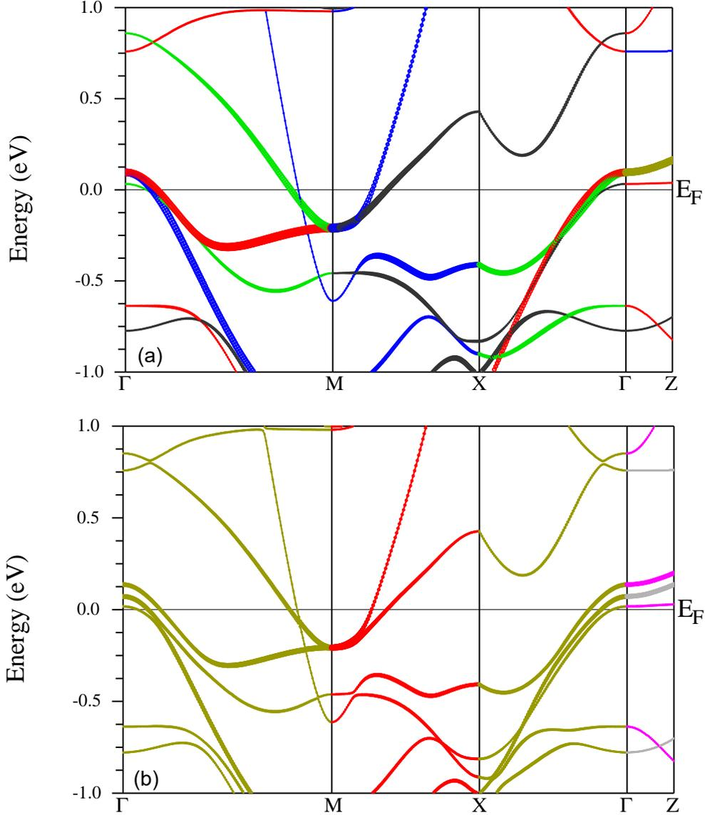
Figure S4. The calculated GGA electronic band structure of  $\text{SrFe}_2\text{As}_2$  in the high-temperature tetragonal phase along several different paths between high symmetry points for the Fe  $d_{xz}/d_{yz}$  orbital character plot (a) in the absence of SOC, and (b) with SOC.
