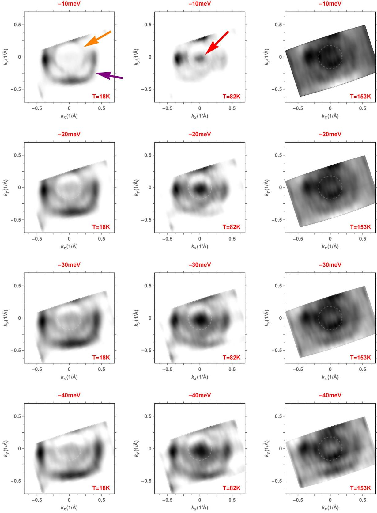
Figure S7. The angle resolved photoemission results for  $\text{Sr}_{0.67}\text{Na}_{0.33}\text{Fe}_2\text{As}_2$  showing the second derivative of the iso-energy ARPES spectra at 18, 82, and 153 K, at -10 meV (first row), -20 meV second row), -30 meV (third row), and -40 meV (last row). The colored arrows point to the corresponding colored parabolic bands in Fig. 6 of the main text.
