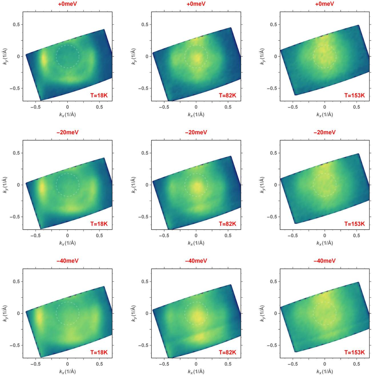
Figure S6. The angle resolved photoemission results for  $\text{Sr}_{0.67}\text{Na}_{0.33}\text{Fe}_2\text{As}_2$  for the iso-energy ARPES spectra for three different temperatures, 18, 82 and 153 K, at the Fermi level (first row), -20 meV (second row), and -40 meV (third row).
