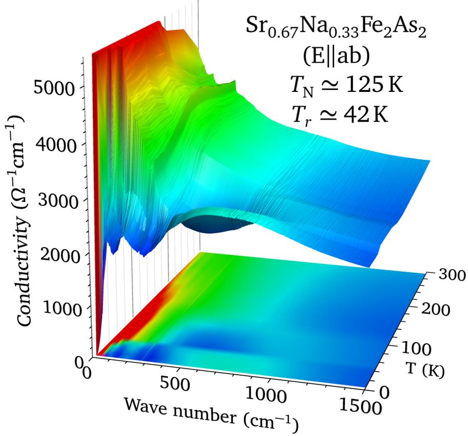
Figure S2. The real part of optical conductivity of  $\text{Sr}_{0.67}\text{Na}_{0.33}\text{Fe}_2\text{As}_2$  in the infrared region for light polarized in the  $ab$ -planes shown as a surface plot, as well as a projection onto the temperature versus wave number plane.
