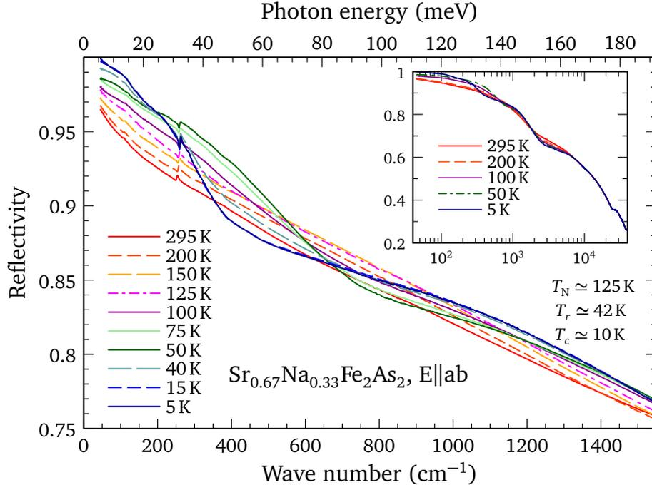
Figure S1. Temperature-dependent reflectivity of  $\text{Sr}_{0.67}\text{Na}_{0.33}\text{Fe}_2\text{As}_2$  in the infrared region for light polarized in the Fe-As planes. Inset: the reflectivity in the high-frequency range at high and low temperatures.
