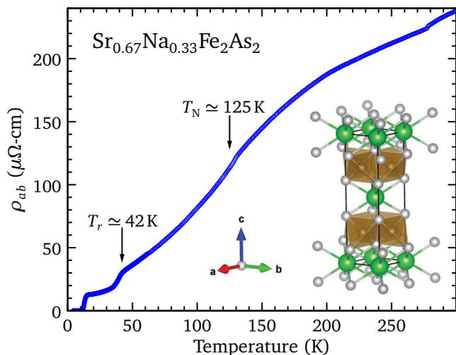
Figure 1. The temperature dependence of the in-plane resistivity for  $\text{Sr}_{0.67}\text{Na}_{0.33}\text{Fe}_2\text{As}_2$  with inflection points at  $T_N \simeq 125$  K and  $T_r \simeq 42$  K; the resistivity at room temperature has been adjusted to match the optical conductivity in the zero-frequency limit. Inset: The generic unit cell in the high-temperature tetragonal phase for the 122 materials.
