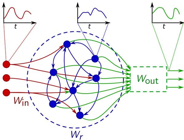
FIG. 1. High-level view of a reservoir computer. Each node may have three kinds of connections: connections to other nodes in the network ( $W_r$ , blue), connections to the overall input ( $W_{in}$ , red), or connections to the output ( $W_{out}$ , green). Note that the internal connections may contain cycles. When the RC is used to perform forecasting, the output on the right side is connected to the input on the left side, allowing the RC to run autonomously with no external input.
